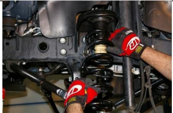
Carefully lower front axle enough to remove front springs.
