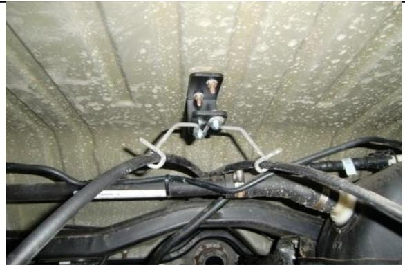
Install provided brake line extension bracket and hardware.
