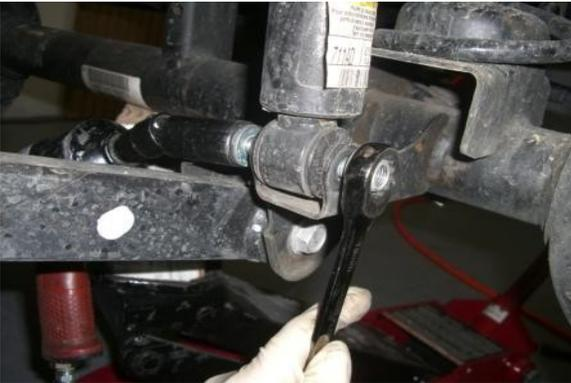
Disconnect and remove front lower shock hardware.
