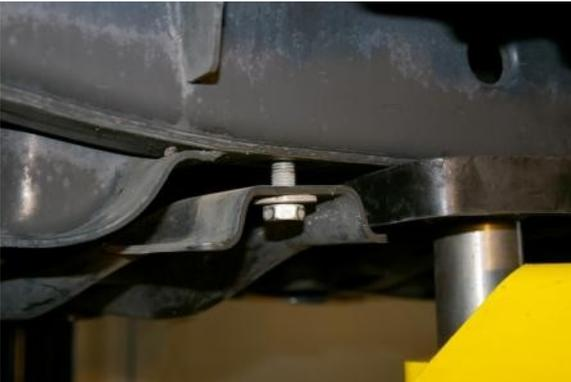
Remove (2) front transfer case skid plate bolts.
