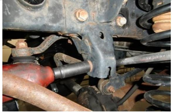
Support front axle and remove upper track bar bolt.
