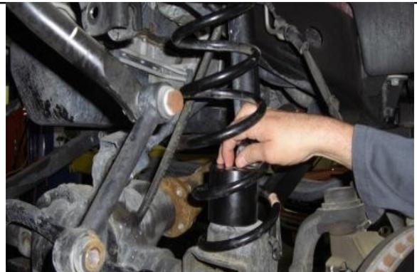
Install new springs/bump stops extensions simultaneously.
