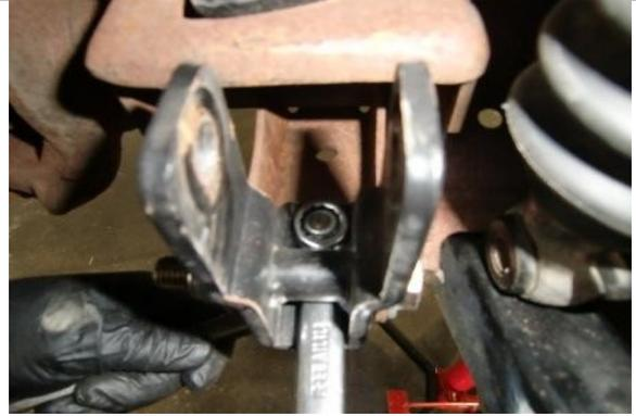
Install front lower shock extensions and torque to spec
