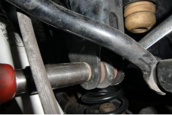
Slightly lift rear axle and remove upper track bar bolt.
