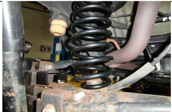
Install new coil springs and OE isolators and raise axle.
