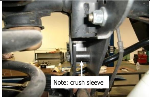
Install new upper track bar bracket with provided hardware.
