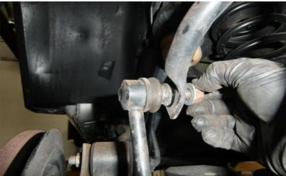
Disconnect and remove rear sway bar end links. Save these links as they will be used on the front sway bar.
