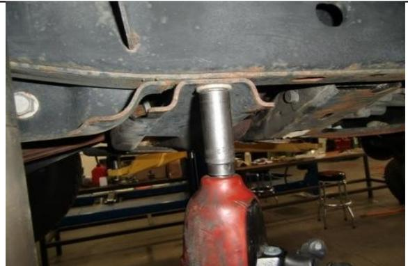
Reinstall front transfer case skid plate bolts.
