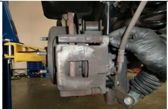
Reinstall rear brake calipers and torque to spec.
