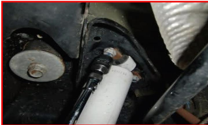
Loosen but do not remove all trailing arms at the frame and axle. Loosen but do not remove the track bar at the frame. Remove the track bar at the axle. Let hang out of the way.
