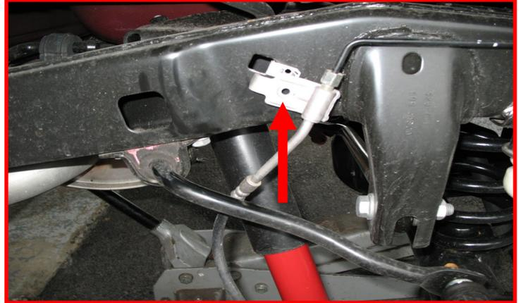
Remove the ABS harness clips from the axle and frame rail. Let hang out of the way.
