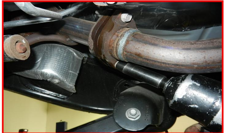
Locate the Y-pipe clamp behind the transmission cross member and loosen using a 15mm socket. Locate the line up tab on the Y-pipe and grind flush with the pipe. This allows the pipe to be slid into the rest of the exhaust once the spacers are installed.
