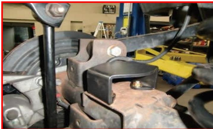
Install the ReadyLIFT rear springs using the factory isolator. Raise the axle up enough to hold the springs in place. Install the provided shocks with the factory hardware. Torque the upper to **35 ft-lbs**. Do not tighten the lower at this time.
