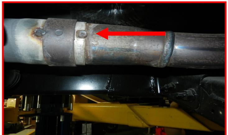
Install the spacers into the exhaust system between the down tubes and Y-pipe using the supplied hardware. The longer of the two goes on the passenger side and shorter on the driver side. Torque the spacer bolts to **45 ft-lbs** and the clamp to **70 ft-lbs**.
