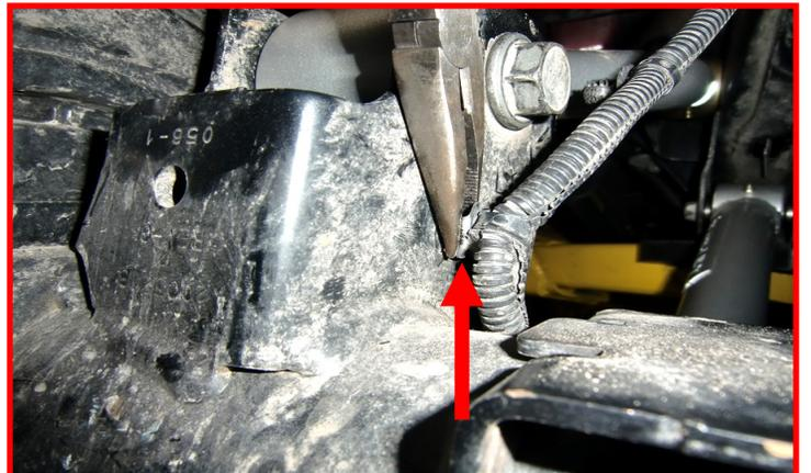
Locate the E-brake cables above the axle and remove the bracket from the body tub. Let hang out of the way.
