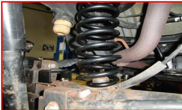
Install the ReadyLIFT E-brake bracket to the tub using the factory hardware. Install the E-brake bracket to the ReadyLIFT bracket using the provided hardware. Torque all to **5 ft-lbs**.
