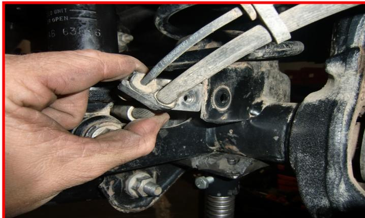
Remove the lower shock hardware at the axle.
