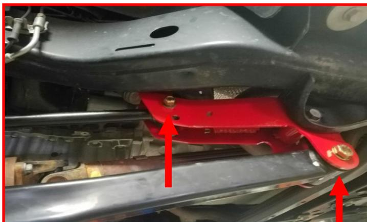
Support the axle with a suitable jack. Remove the front brake line brackets at the axle and frame rail. Let hang out of the way. Remove the vent tube from the driver side spring mount. Let hang out of the way.
