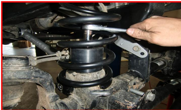
Install the ReadyLIFT 10" sway bar end links to the axle and sway bar using the factory hardware at the sway bar and the provided hardware at the axle. Make sure to use the "fender" washer to the outside of the end link. Do not tighten at this time.
