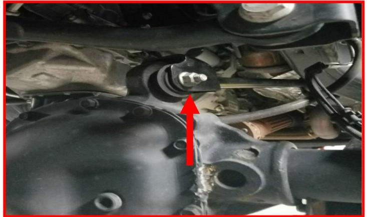
Loosen but do not remove the lower control arm bolts at the axle.
