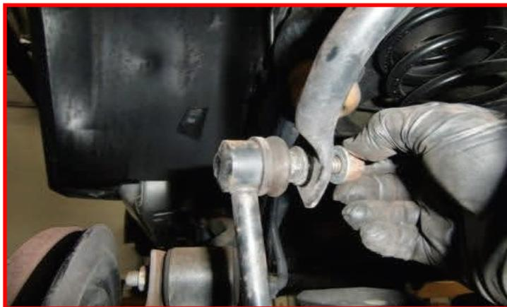
Lower the axle enough to remove the springs from the vehicle. Be careful to not overextend the brake lines and ABS harness.
