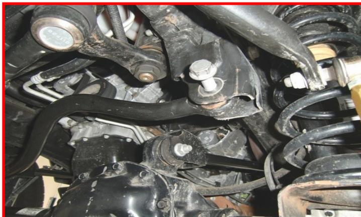
Lower the axle low enough to remove the front springs.
