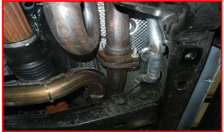
Remove the 4 bolts using a 13mm socket to disengage the Y-pipe from the down tubes. Discard bolts as they will not be re-used.
