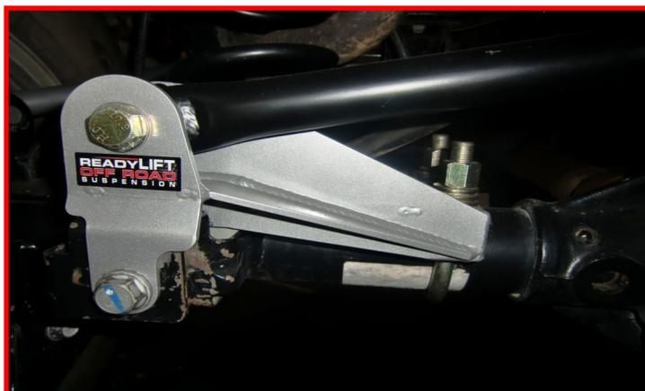
Install the ReadyLIFT rear bump stops using the provided hardware. Torque to **15 ft-lbs.**
