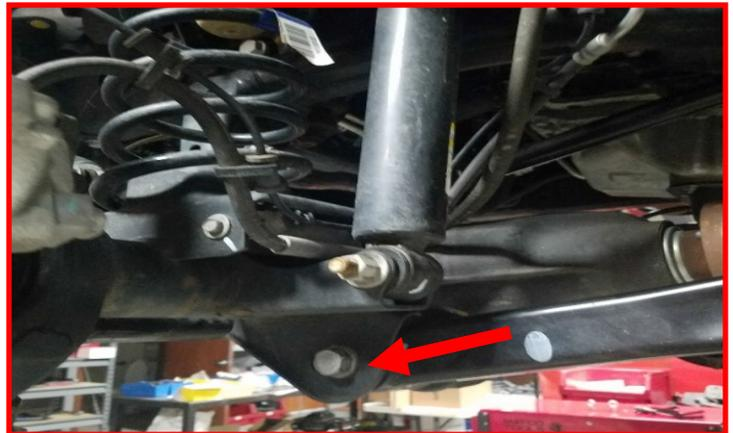
Locate the upper control arms where they meet the frame. Remove the bolt that holds the heat shield to the frame.
