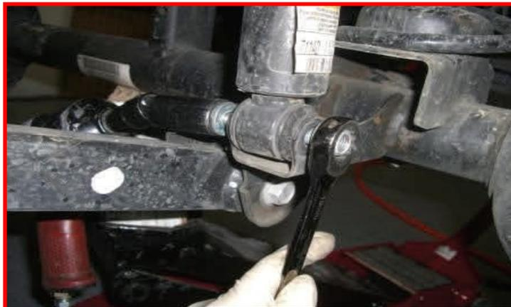
Remove the front sway bar end links from the axle and sway bar. Mark the front driveshaft to pinion location. Remove the front driveshaft hardware. Let hang out of the way.
