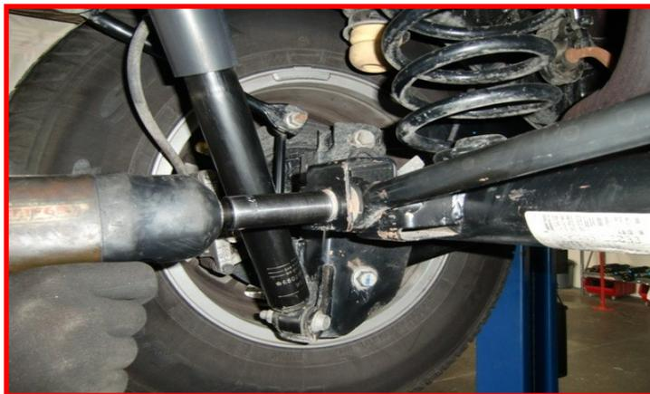
Remove the sway bar end links from the axle and the sway bar.
