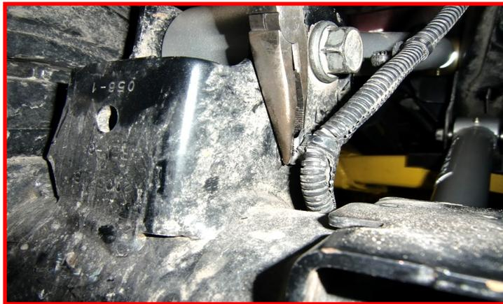
Install the ReadyLIFT rear brake line bracket to the frame rail using the factory hardware. The bracket is offset and will end up under the frame rail when installed properly. Install the factory brake line bracket to the ReadyLIFT bracket using the provided hardware. Torque all to **5 ft-lbs**.
