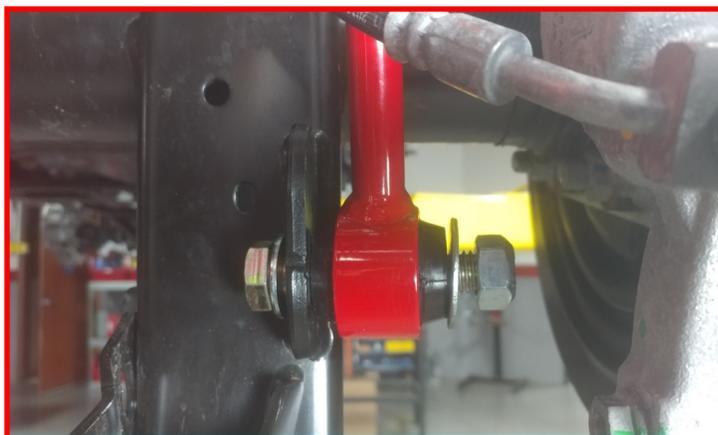
Install the ReadyLIFT rear sway bar end links at the sway bar using the factory axle side hardware at the sway bar. Torque to **45 ft-lbs**.
