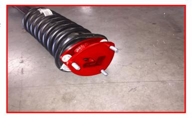
Raise the assembled strut into place, and thread the provided M10 nuts on by hand. Do not tighten at this time.
