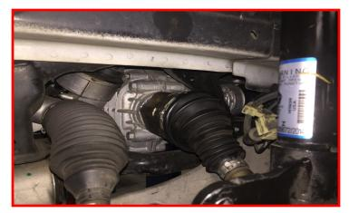
Remove the upper strut hardware. Make sure to hold the strut assembly from falling out of the vehicle. A helper is recommended for removal. Measure down 3/8" on the upper strut mount studs. Using a suitable cut-off tool, trim the studs down to this length for fitment of the strut spacer.
