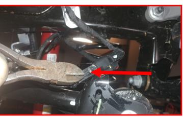
Remove the front sway bar end link from the sway bar. Discard as it will not be reused.
