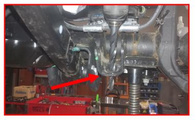
Install the ReadyLIFT front shock extension using provided  $1/2'' \times 1.25''$  bolt, washers, and nut. Use the factory hardware to line up the holes while tightening the 1/2'' hardware. Once tight, remove the factory hardware.
