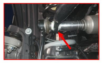
Remove the front lower shock from the axle.
