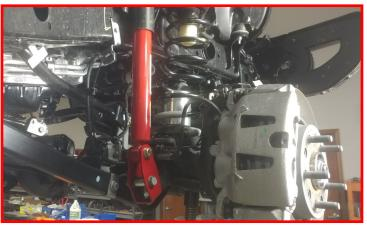
Install the factory rear end links to the sway bar and axle using the factory hard-ware. Torque to 45 ft-lbs.
