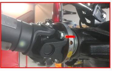
Remove the front drive shaft from differential.
