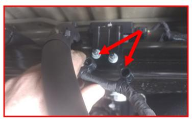
Remove the e-brake cable clamp from the body. Let cables hang. Make sure they are not resting on the locker harness that lays across the frame cross member. When lowering the axle, these cables will become taut and can pinch on the harness.
