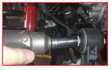
Mark the front drive shaft to pinion flange for reinstallation later.
