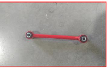
Install the ReadyLIFT sway bar end link to the axle using the provided 1/2" x 2.75" bolt, fender washer, flat washer and nut. Make sure to have the fender washer to the outside of the end link. Do not tighten at this time.
