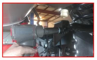
Lower the axle enough to remove the stock spring and rubber isolator. Install the ReadyLIFT spring and factory isolator. Raise the axle enough to hold the springs in place.
