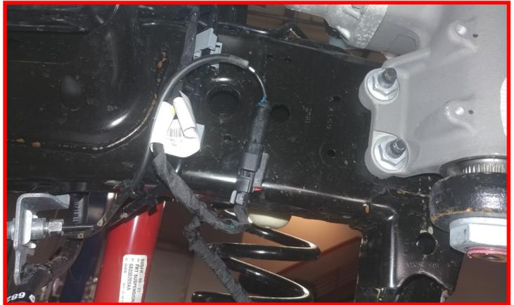
Install the wheels and lower the vehicle to the ground. Install the front drive shaft making sure to line up the previous mark using a **drop of thread locker and factory hardware**. Torque to **40 ft-lbs**.
