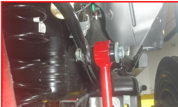
Install the ReadyLIFT sway bar end link to the axle using the provided **1/2" x 2.75" bolt, fender washer, flat washer and nut**. Make sure to have the fender washer to the outside of the end link. Do not tighten at this time.
