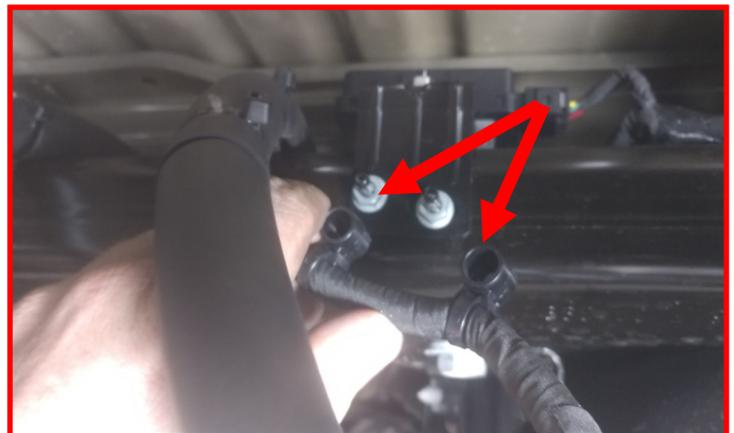
Remove the e-brake cable clamp from the body. Let cables hang. Make sure they are not resting on the locker harness that lays across the frame cross member. When lowering the axle, these cables will become taut and can pinch on the harness.
