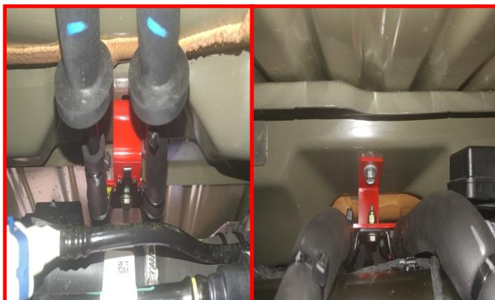
**ELECTRIC LOCKER EQUIPPED MODELS ONLY:** Connect the electrical connector to the pumpkin and run the harness next to the diff vent tube. Clip all remaining clips to the diff vent tube.
