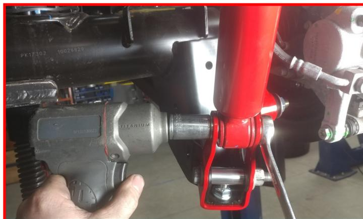
Install the brake line bracket to the axle using the **factory hardware**. Torque to **5 ft-lbs**.
