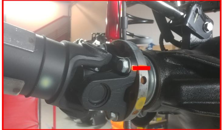
Remove the front drive shaft from differential.
