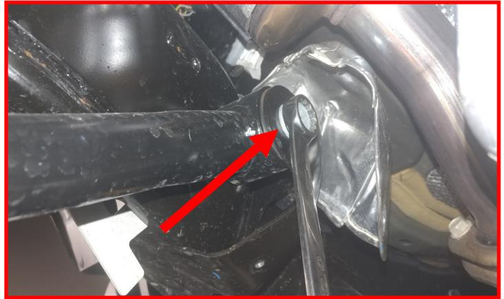
Loosen but do not remove the front upper control arms at the axle.
