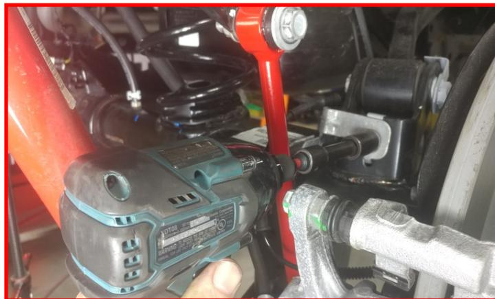
Install the ReadyLIFT brake line bracket to its corresponding side using the provided **1/4" x .75" bolt, washers and nut**. Gently rotate/bend the metal brake line until you can line up the locking tab and bolt hole. Install using the **factory hardware**. Torque all to **5 ft-lbs**.
