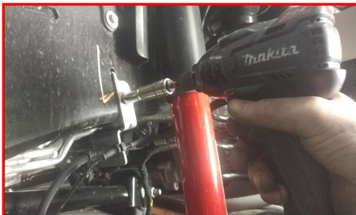
Remove the front brake line bracket at lower control arm.
