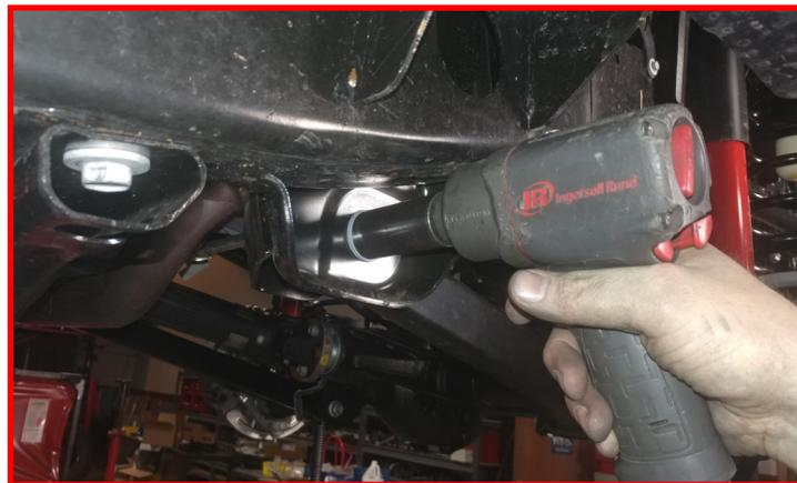
Remove the lower heat shield bolt from the front upper control arm pocket at the frame.
