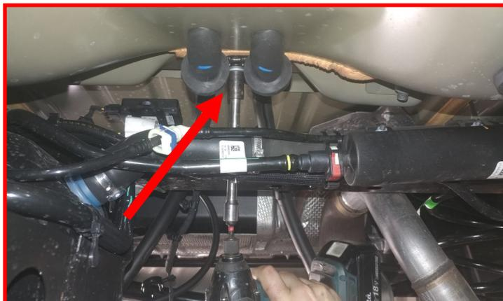
Remove the rear brake line bracket at the axle and frame rail.
