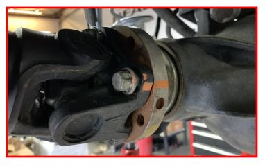
Remove the front drive shaft from differential.
