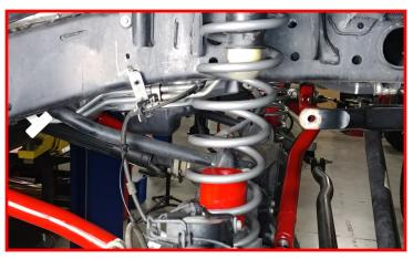
Install the 10" replacement end links to the sway bar using supplied M12-1.25 serrated flange nut on the sway bar.
