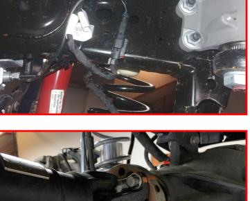
Install the wheels and lower the vehicle to the ground. Torque the lug nuts to the wheel manufacturer specs. Jounce the vehicle a few times to settle the suspension to the new ride height. Torque the upper control arms to 110 ft-lbs, lower control arms and track bar hardware to 135 ft-lbs, and shock and sway bar end link hardware to 50 ft-lbs. Reinstall the upper control arm heat shields. Torque to 5 ft-lbs.
