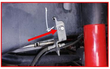
Remove the front brake line bracket at lower control arm.
