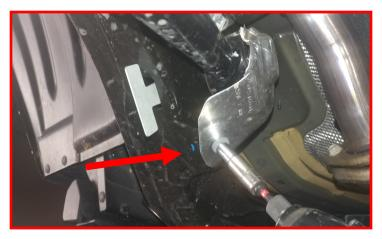
Gently bend the heat shield out of the way and loosen but do not remove the front upper control arm bolts.
