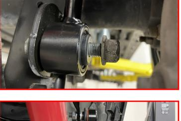
Install the brake line bracket to the axle using the factory hardware. Torque to 5 ft -lbs.
