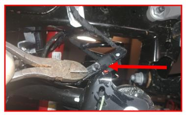
Remove the sway bar end links from the axle. Save the hardware.
