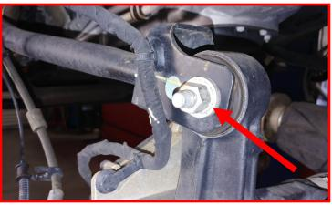
Loosen the front lower control arm hardware at the frame. Do not remove at this time.
