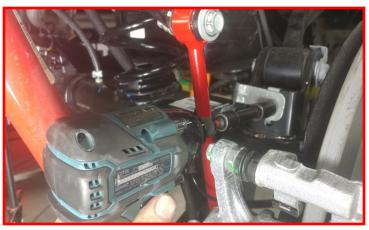
Install the ReadyLIFT brake line bracket to its corresponding side using the provided  $1/4'' \times .75''$  bolt, washers and nut. Gently rotate/bend the metal brake line until you can line up the locking tab and bolt hole. Install using the factory hardware. Torque all to 5 ft-lbs.
