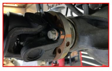
Remove the front drive shaft from differential.
