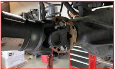
Install the wheels and lower the vehicle to the ground. Torque the lug nuts to the wheel manufacturer specs. Jounce the vehicle a few times to settle the suspension to the new ride height. Torque the upper control arms to 110 ft-lbs, lower control arms and track bar hardware to 135 ft-lbs, and shock and sway bar end link hardware to 50 ft-lbs. Reinstall the upper control arm heat shields. Torque to 5 ft-lbs.
