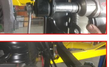
Remove the rear lower control arms at the axle and frame. Retain factory hardware.
