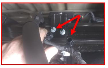
Remove the e-brake cable clamp from the body. Let cables hang.
