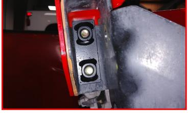
Slide rear track bar bracket crush sleeve into factory track bar bracket and install provided 14mm bolt, washers and locking nut through factory track bar bracket bolt hole. Tighten and torque to 110 ft-lbs.
