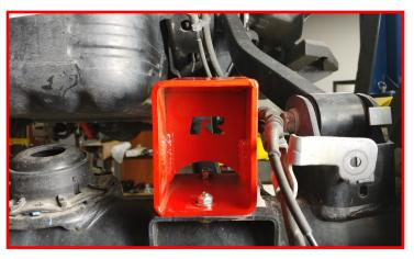
Locate replacement rear track bar bracket and slide over factory axle bracket. Mark center for two 1/2" holes on the outboard side of bracket. Using the appropriate tools drill 1/2" holes through the factory bracket.
