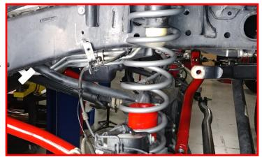
Install the 10" replacement end links to the sway bar using supplied M12-1.25 serrated flange nut on the sway bar.
