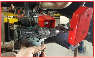
Install provided nut plate to backside of drilled holes. Install supplied 1/2" bolts and washers through drilled holes into nut plate being sure to apply thread locker before tightening. Torque to 90 ft-lbs.
