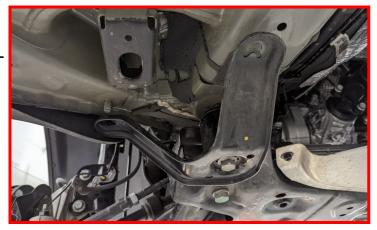
Loosen, but do not remove the front subframe nuts.
