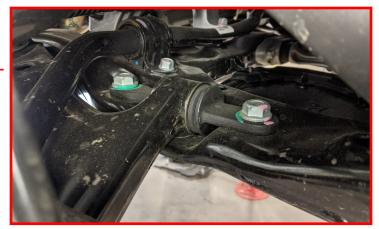
Remove one of the bolts. Install one lower control arm spacer in between the control arm and the subframe. Install the M14x80mm and washer into the threaded hole on the bottom of the subframe. Bolt should be pointing up and coming through the hole in the control arm bracket. Tighten bolt to 100 lb-ft. install nut on top side, but do not tighten. Repeat for the other side hole on the control arm bracket. Tighten both nuts to 100 lb-ft.
