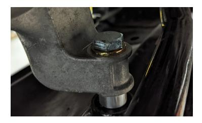
Locate the ReadyLIFT front strut extension. Install to the top of the strut using the factory hardware. Torque to 30 ft-lbs. Set assembly aside and move on to next step.
