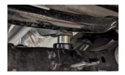
Install ReadyLIFT 1/2" steering gear spacers in between steering gear and subframe using provided M12 bolts and washers.
