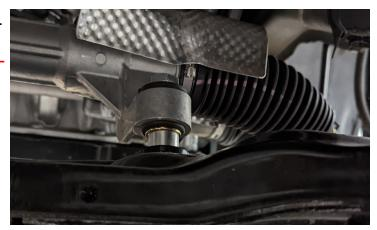
Tighten steering gear hardware down to 50 ft-lbs.
