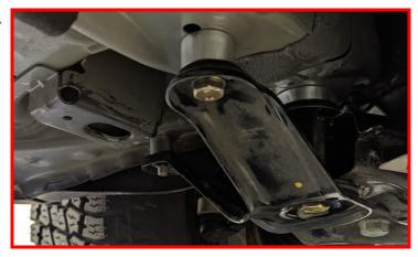
Install the ReadyLIFT front subframe spacer into the front subframe mounts.
