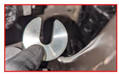
Tighten front and rear subframe hardware to 110 ft-lbs.
