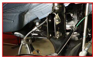
Remove the upper strut hardware. Make sure to hold the strut assembly from falling out of the vehicle. A helper is recommended for removal. Retain Factory Hardware.
