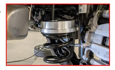
Position the spring spacer with the nipple on the vehicle body.
