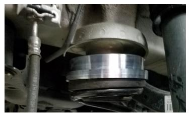
Seat the spring on the lower spring seat. Ensure that the spring is seated correctly against the stop on the lower spring seat.
