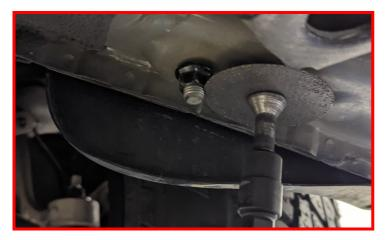
Remove the factory nut and thread the ReadyLIFT subframe auxiliary bracket stud spacer onto the stud that was cut down. Use a 22mm or 7/8" wrench to tighten the spacer down.
