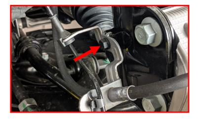
Attach the sway bar end link bracket to the strut assembly. Use provided hardware.
