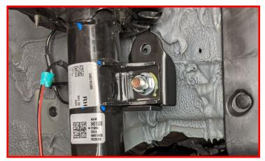
Add the End Link ball joint spacer to the sway bar end link. Attach the sway bar end link to the previous installed bracket with the spacer between the end link and bracket. Use factory hardware.
