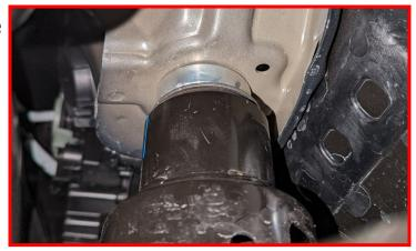
Loosen, but do not remove hardware attaching steering gear to subframe.
