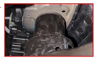
Thread the factory auxiliary bracket nut onto the stud until it bottoms out, leaving it hand-tight. Cut off the length of the stud that is protruding below the nut.
