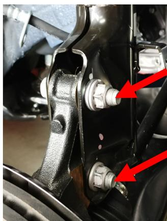
While keeping the lower control arm supported, release the knuckle from the strut body and let hang out of the way. Make sure to not overextend the ABS, brake line, and CV axle. Adjust as necessary.
