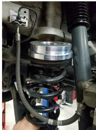
Position the **spring spacer with the nipple** on the vehicle body. The spring seated on the **lower control arm spring isolator**.
