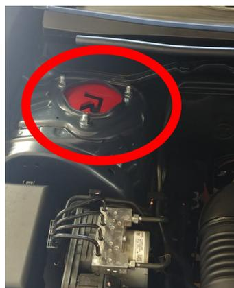
Install the completed strut assembly to the strut tower using the provided M10 flange nuts. Leave loose to aid in installation of the knuckle. A helper is recommended.
