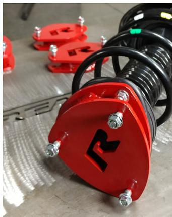
When installed correctly, the **R logo** will be legible through the strut tower when facing the engine compartment from the side that you are on. Passenger side shown. The spacers are offset to the inside and rear of the vehicle to adjust for camber and caster. **THEY MUST BE INSTALLED AS SHOWN.**
