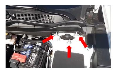
Note: The strut extensions are specific to driver and passenger sides. There is an arrow for correct orientation. D or P for driver and passenger side. Use the alignment pin on the strut assembly to correctly align the strut extension. Use factory hardware to fasten.
