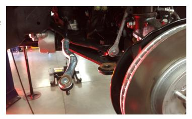
Disconnect the three nuts holding the lower ball joint mount to the lower control arm.
