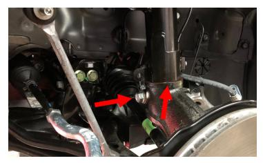
Attach the provided sway bar extension bracket (shown in red) to the strut body using provided M10 hardware.
