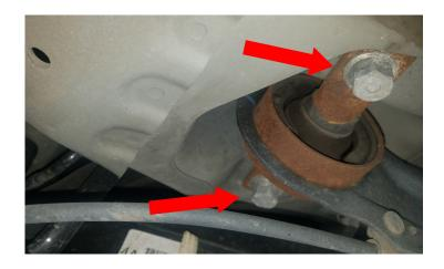
Support the rear suspension cradle with a suitable jack. Remove the cradle brackets. Remove each bracket individually. The rear cradle brackets will use the provided M14x180mm and M8x45mm hardware. Install the included spacers and partially thread the provided hardware to allow the cradle to lower and ease installation of other brackets.
