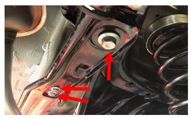
Remove each front cradle bracket and install the remaining cradle spacers (shown in red) using the provided M8x45mm and M14x160mm hardware.
