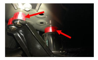
Remove the lower strut bolt.
