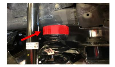
Using the provided M14x90mm hardware, install the provided trailing arm spacer (shown in red) towards the rear of the vehicle between the trailing arm and vehicle body.
