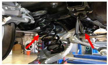
Remove the two bolts holding the upper shock mount to the vehicle body and remove the shock from the vehicle.
