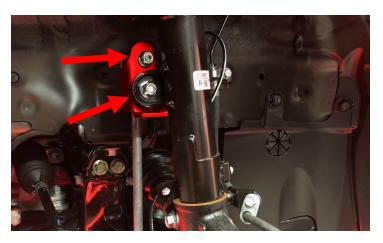
Pry down on the lower control arm to re-install the three lower ball joint studs.
