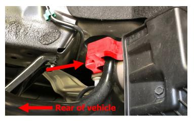
Attach the shock absorber to the lower mount. Thread in bolt, but do not tighten at this time.
