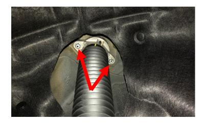
Install the provided shock extension (shown in red) between the vehicle body and the shock absorber.
