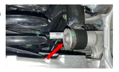
Install sway bar links to spindle. Do not tighten at this time.
