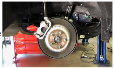
Un-bolt the sway bar end links at the control arm. You may do this on both sides to facilitate movement. Remove the shock bolt at the control arm.
