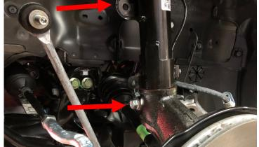
Open the hood. Remove the hardware attaching the strut assembly to the body.
