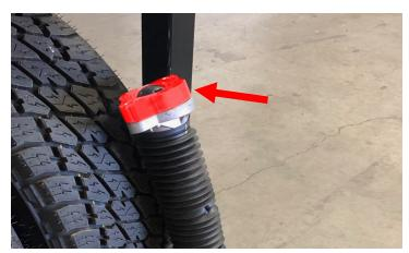
Install the provided coil spring spacer (shown in red) on top of the rubber coil spring insulator.
