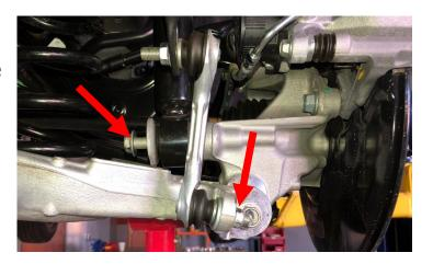
Remove the trailing arm bolts from the frame of the vehicle.
