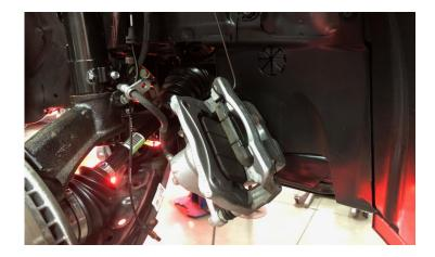
Disconnect the outer tie rod end from the knuckle. It may be necessary to strike the tie rod boss with a hammer to dislodge the taper.
