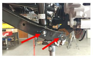
Remove the strut assembly from the vehicle and let the control arm hang.
