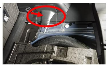
Remove the strut nuts and set aside.
