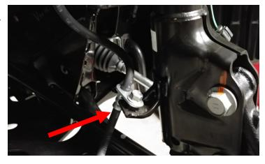
Loosen but do not remove the sway bar end link from the sway bar.
