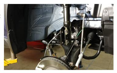
Remove the upper strut hardware. Make sure to hold the strut assembly from falling out of the vehicle. A helper is recommended for removal.
