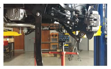
Locate the ReadyLIFT strut extension. Install using the factory hardware. You will have to start each nut before tightening fully. Run each nut down in an alternating pattern until you can torque them down. Torque to 30 ft-lbs.
