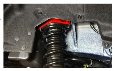
Support the rear subframe assembly. Remove the 2 bolts holding cradle retainer to the body and the bolt holding the trim molding to the retainer.
