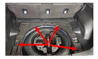
Remove these clips and set the foam pieces aside. Remove the strut covers by pulling upwards at the trunk area, then pushing down at the plastic cover, and set aside.
