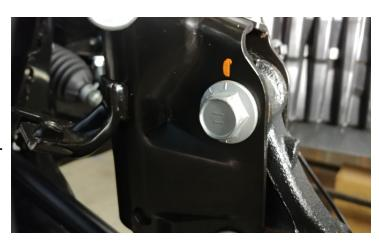
Re-attach brake line bracket in original location using factory hardware. Torque to 5 ft-lbs.
