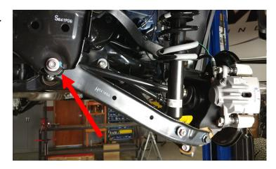
Support the strut and lower control arm, remove the lower strut and knuckle bolts. Lower the control arm down, while holding the strut. Remove the strut from the vehicle. A helper is recommended to hold the strut from falling.
