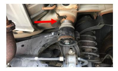
Install the cradle bracket spacer between the retainer and the body, and thread in the (2) provided M10 bolts and OE trim to retainer bolt.
