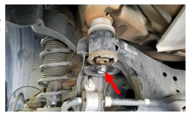
Raise cradle and tighten all bolts. Torque cradle bolts to 120 ft-lbs.
