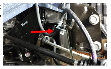
Remove the ABS harness clip at the strut body. Let hang out of the way.
