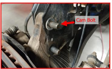
Reinstall the brake line bracket to the strut body using the factory hardware. Torque to 5 ft-lbs.
