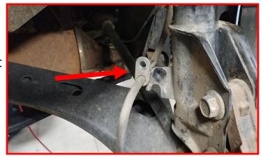
Remove the ABS wire from the strut body. Let hang out of the way.
