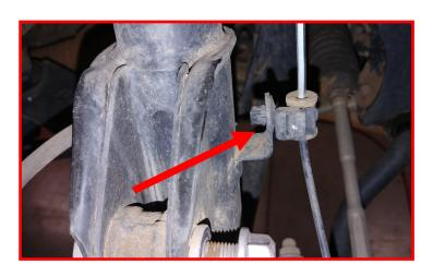
The cam bolt has lines that correspond to a notch on the strut body (paint marked for picture clarification). You will rotate the cam bolt until the lines are facing the inside of the vehicle. Line up the last line with the notch. This sets max negative camber. Torque both bolts to 95 ft-lbs. Final adjustment and torque to be set by the alignment tech.
