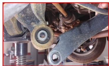
Reinstall the sway bar to the subframe using the factory hardware. Torque to 15 ft-lbs. Install the wheels and lower the vehicle to the ground. Torque the lug nuts to the wheel manufacture's specs. Jounce the vehicle to get it to settle to the new ride height. Torque the upper strut hardware to 30 ft-lbs. Install the strut covers. Torque all the upper, lower control arm and lower strut hardware to 95 ft-lbs, and sway bar end link hardware to 35 ft-lbs.
