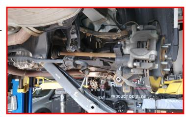
Install the ReadyLIFT strut extension using the factory hardware. You will have to start each nut before tightening fully. Run each nut down in an alternating pattern until you can torque them down. Torque to 30 ft-lbs.
