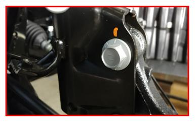
Install the front wheels and lower the vehicle to the ground. Torque the lug nuts to the wheel manufacturers specs. Jounce the front end to settle the suspension. Torque the upper strut spacer to 30 ft-lbs.
