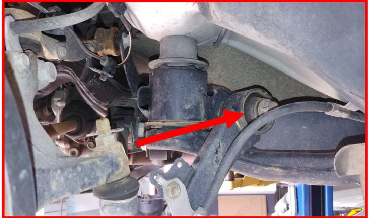
Remove the front lower control arm bolt at the knuckle. Let the control arm hang out of the way. This is for access to the rear lower control arm bolt removal.
