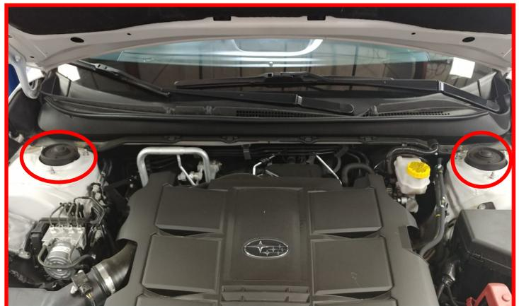
Locate the ReadyLIFT front strut extension. These are driver and passenger side specific and are etched with a D and P. Passenger side shown. Install to the top of the strut using the **factory hardware**. Torque to **30 ft-lbs**.
