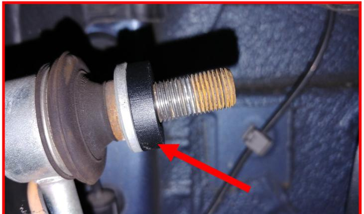
Install the factory end link to the ReadyLIFT bracket using the **factory hardware**. Torque the bracket and end link to **45 ft-lbs**.
