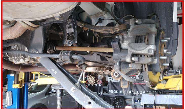
Locate the ReadyLIFT strut extension. Install using the **factory hardware**. You will have to start each nut before tightening fully. Run each nut down in an alternating pattern until you can torque them down. Torque to **30 ft-lbs**.
