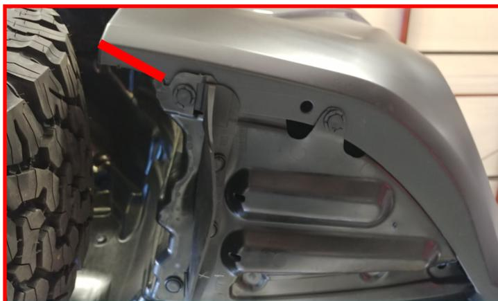
Remove the mud flap/rock guard on the rear of the fender well, or trim to fit. You can easily trim all parts of the bumper cover and plastic with a razor knife. Test clearance by turning the wheel full lock while pulling forward and reverse. Trim as necessary until the tire does not rub anymore.
