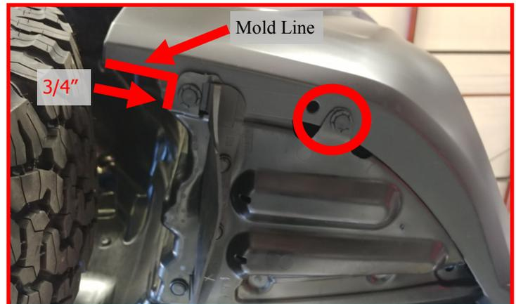
Once this is done, tuck the plastic line up above the bumper cover minus the one tab in the middle (circled in red). Once the plastic liner is in place, drill through the bumper cover in the two mounting locations using a  $1/2$ " drill bit. Install the previously removed rivets. On the leading edge of the bumper cover there will be a tab that is left unused. You can trim this off as shown.
