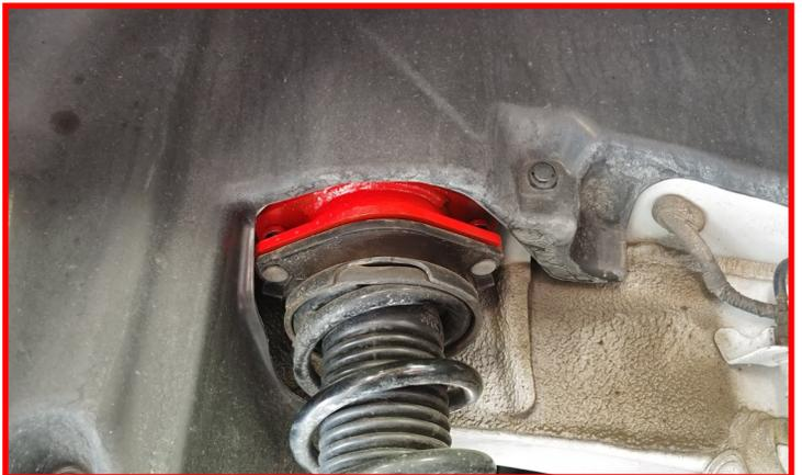
Raise the lower control arm into place and install the **lower strut hardware**. Do not tighten at this time. Use the jack and raise the lower control up to set pre load on the strut. Install the lower **knuckle bolt**.
