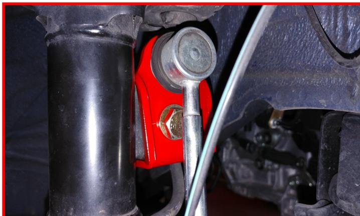
Install the front wheels and lower the vehicle to the ground. Torque the lug nuts to the wheel manufacturers specs. Jounce the front end to settle the suspension. Torque the upper strut spacer to **30 ft-lbs**
