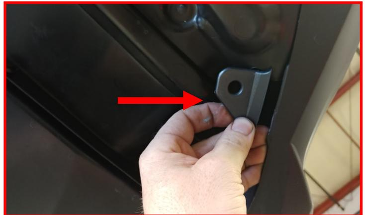
The inside edge clip holes can now be lined up and drilled out. Once done, reinstall using the previously removed clips.
