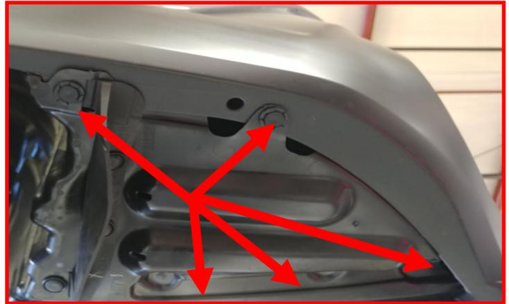
From the edge of the bumper cover closest to the wheel well, measure to the front  $3/4$ " and mark a line as shown. There is a mold line for the forward cut you can follow. Use a suitable cutting tool and trim this lip off. You will be removing the last mounting hole and trimming this area allows the plastic to slide forward.
