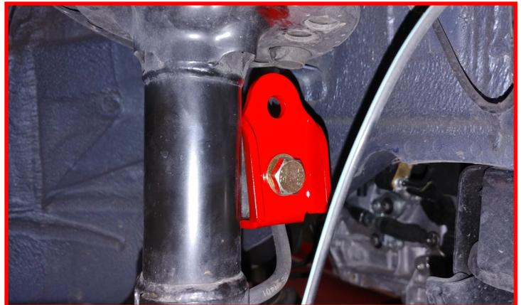
Install the **1/4" thick spacer** washer onto the end link.
