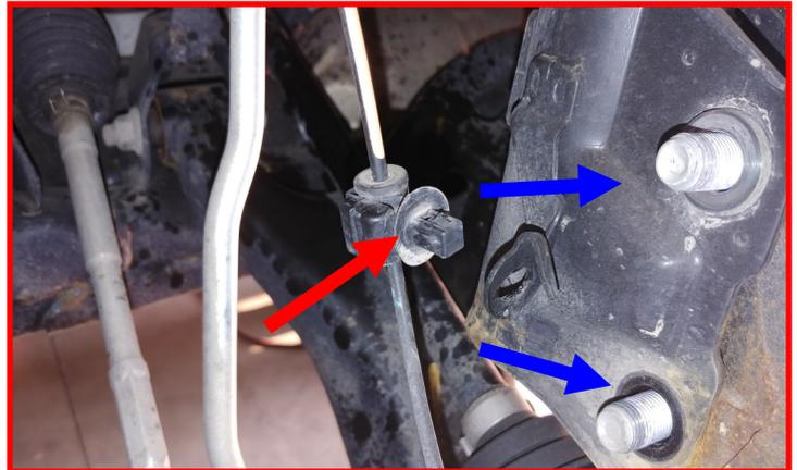
While keeping the lower control arm supported, release the knuckle from the strut body and let hang out of the way. Make sure to not overextend the ABS, brake line, and CV axle. Adjust as necessary.
