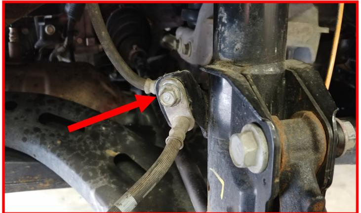
Install the ReadyLIFT sway bar bracket to the strut using the provided **M12 bolts, washers, and nuts**. Do not tighten at this time. If you have not started the opposite side of the vehicle at this time, you may not be able to line the sway bar up until the opposite side is released.
