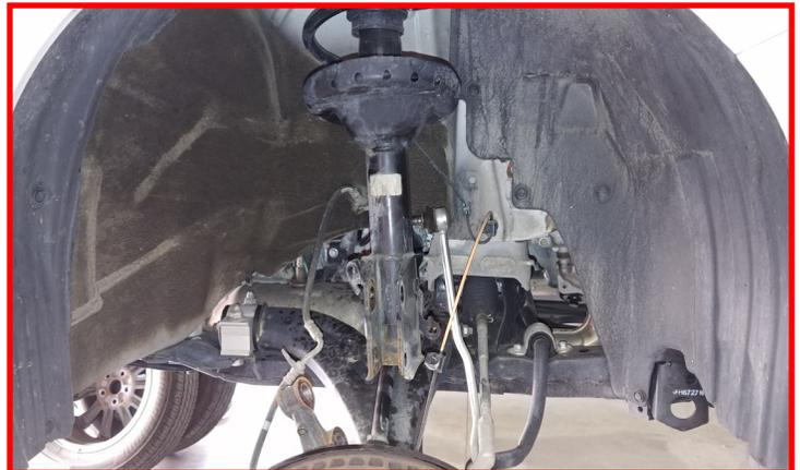
Remove the upper strut hardware. Make sure to hold the strut assembly from falling out of the vehicle. A helper is recommended for removal.
