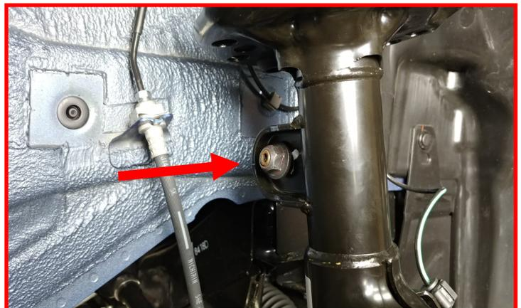
Remove the brake line bracket at the strut body. Let hang out of the way. Note how the brake line is run from the underside of the strut body. Installation will be changed in a later step.
