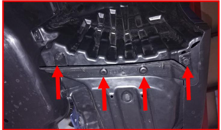
Remove all remaining **plastic push clips** from the inner fender liner. There are 4 clips. Save all clips. Note that the liner sits under and over the bumper cover. This will be changed later. Remove 1 **plastic push clip** from the lower skid plate and bumper cover.
