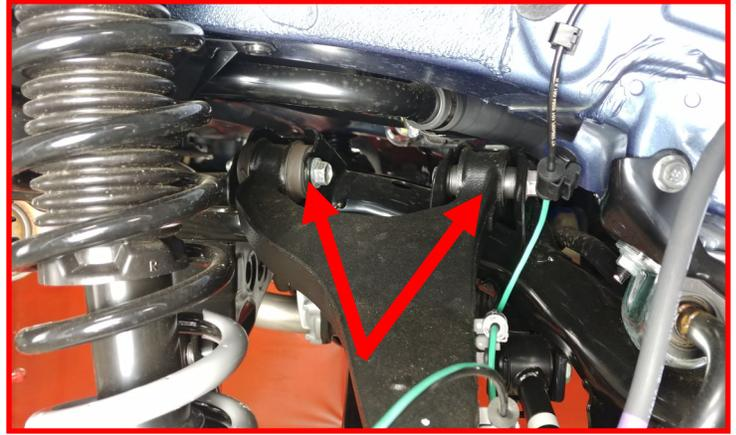
Loosen but do not remove the front lower control arm bolts.
