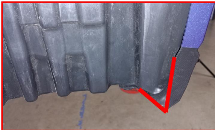
Locate the "mud flap" on the back of the wheel well. This can be trimmed the same as the front bumper cover. Cut straight down to the 90 degree turn, then cut at a 45 degree to the pinch weld. Make sure to cut to the inside of the plastic push clip. The plastic is very easily cut, so take care to not slip. This can be trimmed more if necessary. Test fitment of the wheel and tire combo is recommended and trim as necessary.
