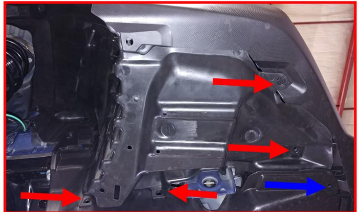
Pull the skid plate down to access the bolt holding the last of the inner fender liner. Remove and discard. Reinstall the **plastic push clip** into the skid plate.
