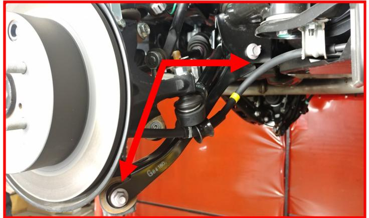
Loosen but do not remove the rear lower control arm bolt at the subframe.
