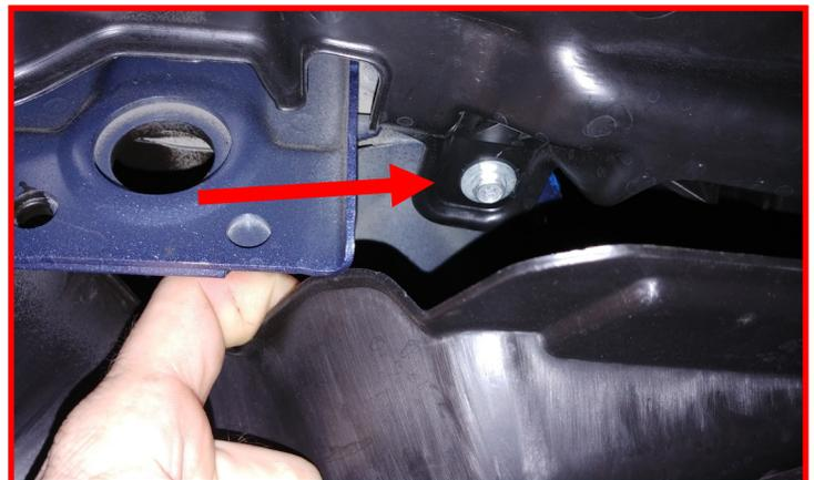
Take the plastic liner and install above the bumper cover. You will see one ear of the bumper cover that originally sits under the liner, this needs to be relocated to the outside of the liner.
