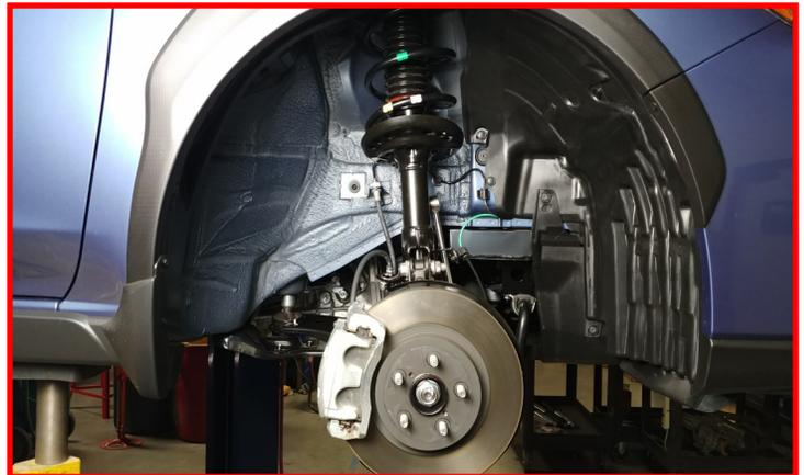
Remove the front sway bar end link at the strut body. This step should be completed on both sides to ease in installation at later steps.
