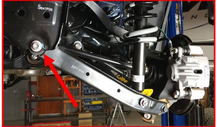
Support the strut and lower control arm, remove the lower strut and knuckle bolts. Lower the control arm down, while holding the strut. Remove the strut from the vehicle. A helper is recommended to hold the strut from falling.
