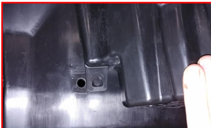
Once the liner is moved forward, use a suitable razor knife and trim the outer bumper cover edge valance. Cut straight down to the 90 degree turn, then cut at a 45 degree to the liner. The plastic is very easily cut, so take care to not slip. This can be trimmed more if necessary. Test fitment of the wheel and tire combo is recommended and trim as necessary.
