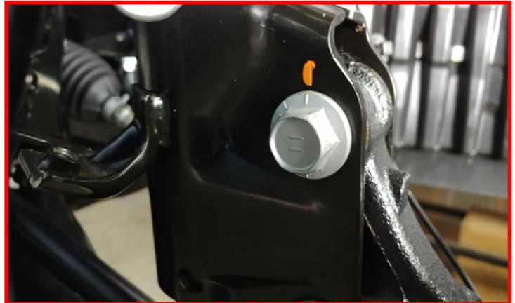
Install the brake line bracket to the strut body. Rotate the brake line bracket as shown. Originally the brake line was bolted from the bottom upwards to the strut, now it will be mounted to the top of the strut body using the **factory hardware**. Torque to **5 ft-lbs**. Make sure to rotate the ferule inside the cut out on the strut body. Refer to disassembly step for reference if needed.
