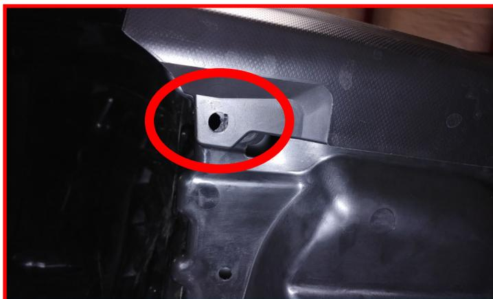
Finish off the liner movement by pushing forward 1". Mark and drill out the new plastic push clip locations. Install the remaining push clips.
