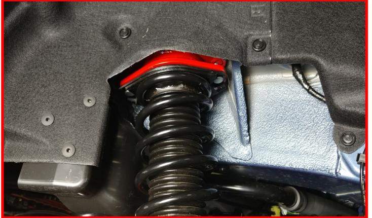
Raise the lower control arm into place and install the **lower strut hardware**. Do not tighten at this time. Use the jack and raise the lower control up to set pre load on the strut. Install the lower **knuckle bolt**. Torque to **95 ft-lbs**.
