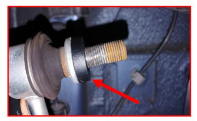
Install the factory end link to the Ready-LIFT bracket using the factory hardware. Torque the bracket and end link to 45 ftlbs.
