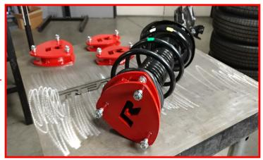
When installed correctly, the R logo will be legible through the strut tower when facing the engine compartment from the side that you are on. Passenger side shown. The spacers are offset to the inside and rear of the vehicle to adjust for camber and caster. THEY MUST BE INSTALLED AS SHOWN.
