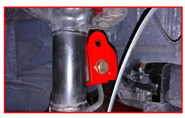
Install the 1/4" thick spacer washer onto the end link.
