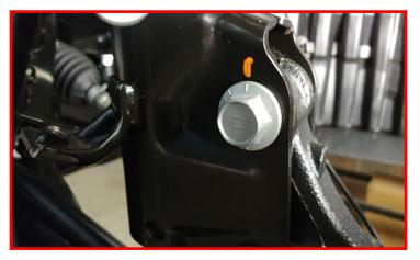
Install the brake line bracket to the strut body. Rotate the brake line bracket as shown. Originally the brake line was bolted from the bottom upwards to the strut, now it will be mounted to the top of the strut body using the factory hardware. Torque to 5 ft-lbs. Make sure to rotate the ferule inside the cut out on the strut body. Refer to disassembly step for reference if needed.
