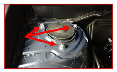
Locate the ReadyLIFT front strut extension. These are driver and passenger side specific and have a D and P etched into the top. Passenger side shown. Install to the top of the strut using the factory hardware. Torque to 30 ft-lbs.
