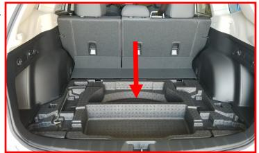
Locate the plastic push clips holding the foam tool holders in place. Remove these clips and set the foam pieces aside.
