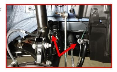
Remove the strut to knuckle bolts. The bolts are specific to upper and lower mounting locations and direction of install. The upper is a cam bolt, while the lower is a standard bolt. Make sure to note their orientation for reinstallation later.
