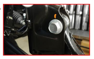
Remove the factory end link from the sway bar. Remove from vehicle and discard.
