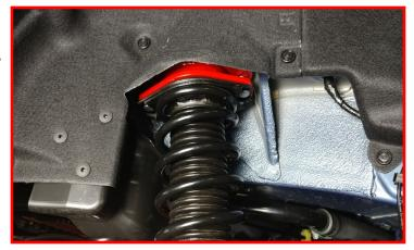
Raise the lower control arm into place and install the lower strut hardware. Do not tighten at this time. Use the jack and raise the lower control up to set pre load on the strut. Install the lower knuckle bolt. Do not tighten at this time.
