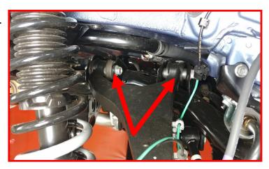
Loosen but do not remove the front lower control arm bolts.
