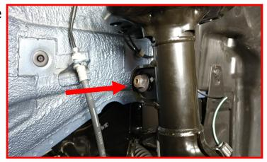
Remove the brake line bracket at the strut body. Let hang out of the way. Note how the brake line is run from the underside of the strut body. Installation will be changed in a later step.
