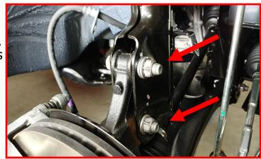
While keeping the lower control arm supported, release the knuckle from the strut body and let hang out of the way. Make sure to not overextend the ABS, brake line, and CV axle. Adjust as necessary.
