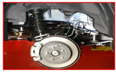
Loosen but do not remove the upper control arm bolts.
