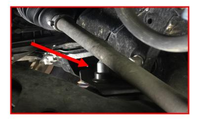
Replace the cradle with the supplied M14 bolts. Apply a drop of thread locker and torque the bolt to 95 ft-lbs. This will provide adequate clearance between the cradle bolt and the CV axle shaft.
