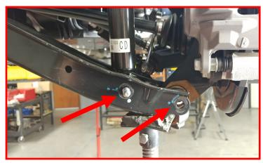
Remove the strut assembly from the vehicle and let the control arm hang.
