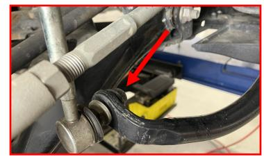
Locate the ReadyLIFT end link. Note that they are drive and passenger side specific. Install the end link to the vehicle using the supplied M10 flange nut. Torque the end link to 45 ft-lbs.
