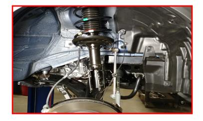
Raise the knuckle up and install into the strut body. Install the cam bolt into the upper hole and the remaining bolt into the lower.
