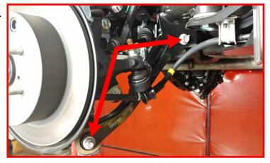
Loosen but do not remove the rear lower control arm bolt at the subframe.
