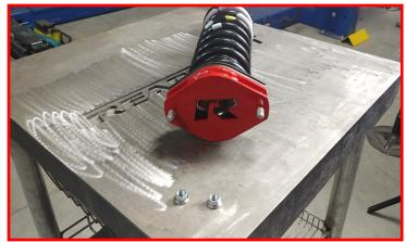
Install the completed strut assembly to the car using the provided M10 flange nuts. Do not tighten at this time. A helper is recommended.
