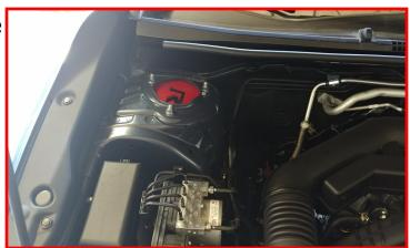
Remove the cradle bolt, one side at a time, and discard.
