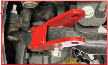
Remove the nut from the tie rod pinch point (18mm). NOTE: Some Ram 2500 models have two bolts on the tie rod pinch point.
