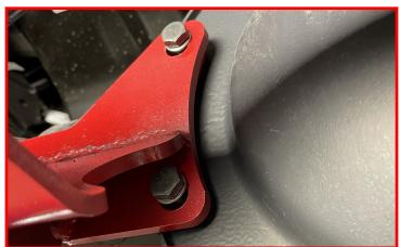
Use a dead blow hammer to install the passenger side ReadyLIFT Tie Rod Bracket to the tie rod using the factory hardware. Make sure the bolts are installed from the bottom.
