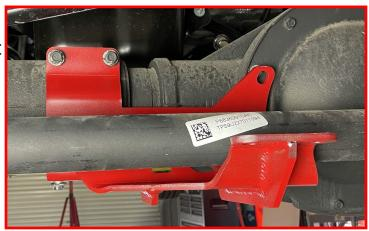
Slide the 0.25" Diff Spacer in-between the diff cover and the Dual Steering Stabilizer bracket. Install using the supplied M8-1.25 x 40mm bolts (13mm) and M8 washers. Do not tighten at this time.
