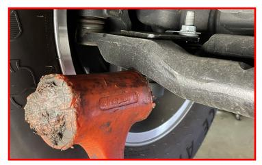
Remove the four M10 bolts (13mm) holding the factory backet onto the axle. Discard the factory stabilizer and brackets
