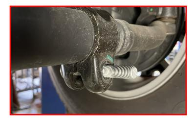
Install the driver side ReadyLIFT U-shaped bracket and crush sleeve outboard of the tie rod pinch point using the supplied M12-1.25 x 80mm bolt (19MM), M12-1.25 nut, and two M12 flat washers. Make sure to install the bolt from back to front.
