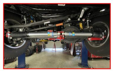
Rotate the wheels from lock to lock and verify all clearances between the tire, frame, and suspension components before lowering the vehicle. Adjust as necessary.
