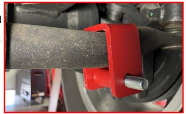
Install the driver side ReadyLIFT bracket onto the tie rod pinch point using the factory nut. Do not tighten at this time.
