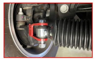
Install the stabilizers damper to the driver side bracket using the provided M12-1.25 x 75mm bolts, M12-1.25 Nuts, and M12 Flat Washers.
