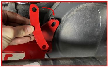
Torque the four M10 steering stabilizer bolts to 40 ft-lb.
