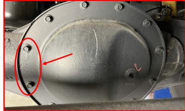
Using the factory hardware, install the ReadyLIFT Dual Steering Stabilizer main body onto the axle. Do not tighten at this time.
