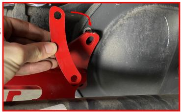
Torque the four M10 steering stabilizer bolts to 40 ft-lb.
