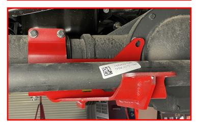
Slide the 0.25" Diff Spacer in-between the diff cover and the Dual Steering Stabilizer bracket. Install using the supplied M8-1.75 x 40mm bolts (13mm) and M8 washers. Do not tighten at this time.
