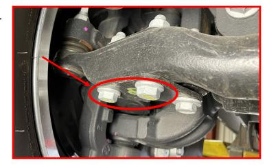
Carefully use a dead blow hammer to shimmy the bracket free.
