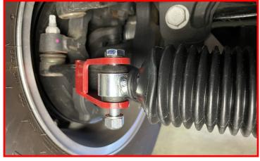
Install the stabilizers damper to the driver side bracket using the provided M12-1.75 x 80mm bolts, M12-1.75 Nuts, and M12 Flat Washers.
