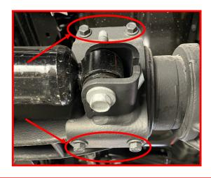
Remove the two M8 factory bolts (10mm) at the 9 o'clock position from the diff cover.
