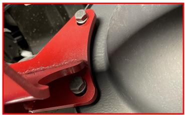
Install the passenger side ReadyLIFT Passenger Stabilizer Mount to the tie rod using the factory hardware. Make sure the bolts are installed from the bottom.
