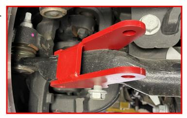
Remove the nut from the tie rod pinch point (18mm). NOTE: Some Ram 2500 models have two bolts on the tie rod pinch point.
