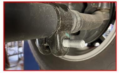
Install the driver side ReadyLIFT U-Bracket and crush sleeve outboard of the tie rod pinch point using the supplied M12-1.75 x 80mm bolt, M12-1.75 nut, and two M12 flat washers. Make sure to install the bolt from back to front.
