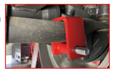
Install the ReadyLIFT Driver Stabilizer Mount onto the tie rod pinch point using the factory nut. Do not tighten at this time.
