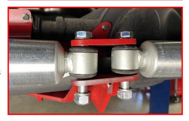
Install the stabilizers damper to the passenger side bracket using the provided M12-1.75 x 80mm bolts, M12-1.75 nuts, and M12 flat washers.
