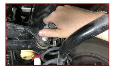
Install new track bar by inserting bushing pivot side into track bar bracket.
