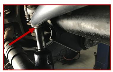
Loosen nut, but do not remove nut completely.
