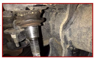
Install track bar onto ball joint and install nut. Tighten factory nut and torque to 185 ft-lbs.
