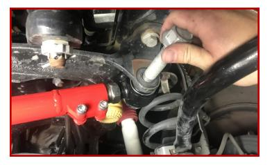
Prior to installing the track bar onto the ball joint, be sure to inspect the ball joint for, tears in the grease boot, excessive wear or otherwise. This would be the optimal time to replace the worn component.
