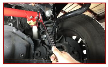
Tighten the (2) 3/8" pinch bolts. While alternating back and forth between the two torque pinch bolts to 55 ft-lbs.
