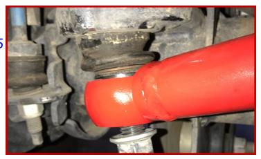
At this point, tighten track bar bracket bolt and torque to 350 ft-lbs.
