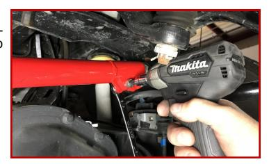
If required, center the steering wheel using the drag link adjustment before driving per factory service manual.
