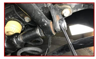
Remove frame side pivot bolt from track bar bracket, and remove complete bar from vehicle.
