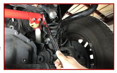
Tighten the (2) 3/8" pinch bolts. While alternating back and forth between the two torque pinch bolts to 55 ft-lbs.
