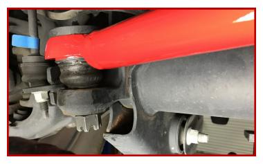
Tighten castle nut and torque to 185 ftlbs].
