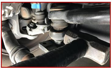
Loosen and remove nut from track bar bracket pivot bolt.
