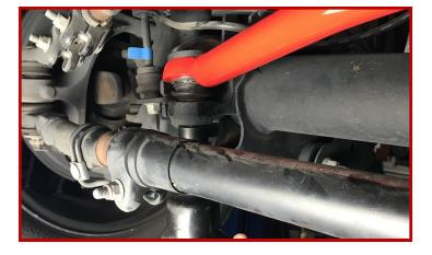
Insuring the castle nut aligns with the predrilled hole, install supplied cotter pin.
