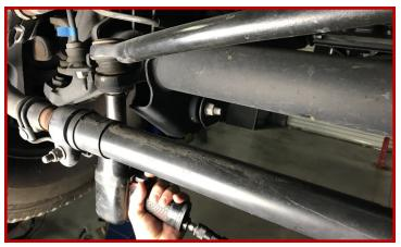
With aid of an appropriate device (i.e. Floor jack, Bottle Jack, Pole jack), apply a lifting force to bottom of the track bar ball joint. Strike side of axle track bar mount to unseat taper using a hammer/Air hammer, as pictured.
