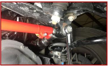
This track bar has been preset at 37", which is the length the average end-user should need.
