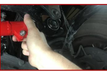
Insert ball joint into taper on the axle and start the nut.
