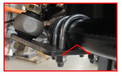
Install the passenger tie rod bracket using the supplied 3/8" U-bolts, 3/8" flat washers, and 3/8" toplock nuts. Place the plate flush against the flat face on the bottom of the tie rod. Do not fully tighten at this time.
