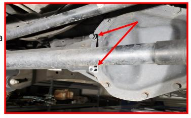
Remove the (2) middle bolts on the driver side differential cover and discard. Install the differential ID tag on the drivers side using the factory hardware.
