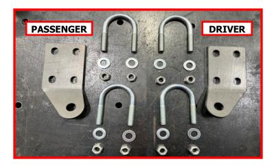
Install the driver tie rod bracket using the supplied 3/8" U-bolts, 3/8" flat washers, and 3/8" toplock nuts. Place the plate flush against the flat face on the bottom of the tie rod. Do not fully tighten at this time.
