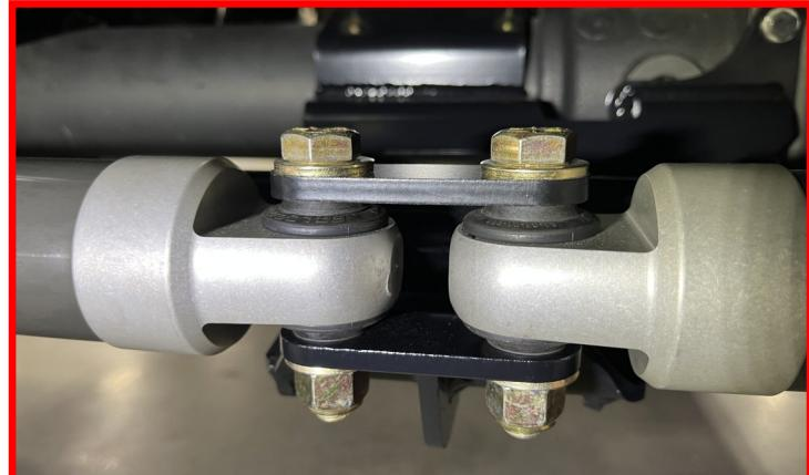
Install stabilizer shaft ends to the tie rod brackets using the **M12 x 65mm bolts, washers and nuts**. The shaft end will sit on top of the angled face (as shown in photo). Do not tighten at this time.
