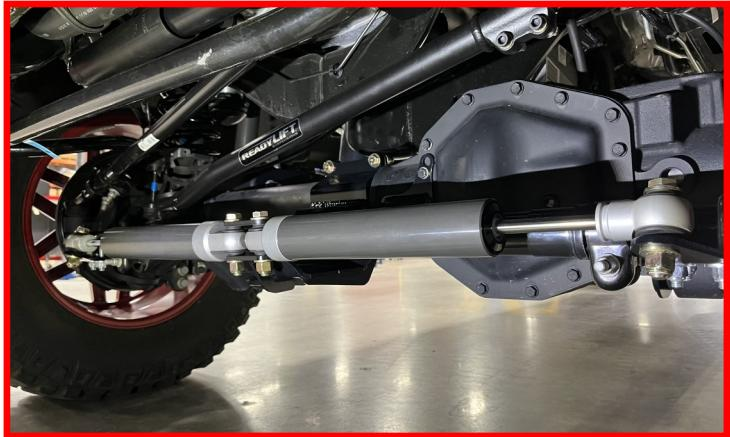
With all the hardware tightened and torqued to spec, complete a full lock to lock sweep of the steering to ensure there are no clearance issues, binding or bottoming out and/or over extension of the stabilizers.
