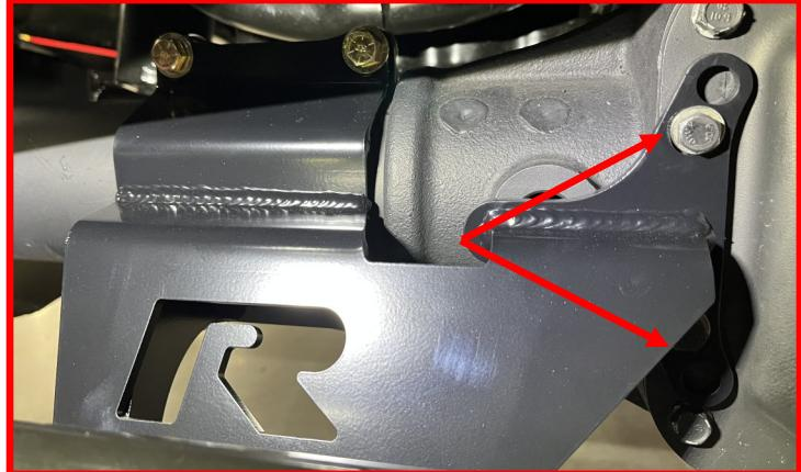
Using the supplied **M10-1.5 x 55mm Hex Head Bolts**, **M10 flat washers** and **M10-1.5 toplock nuts**, fasten the **rear axle bracket** to the **center stabilizer bracket**, clamping both around the axle tube.
