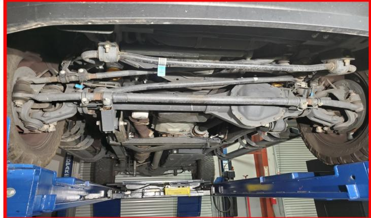
Remove the **(2) middle bolts** on the passenger side of the differential cover and retain the factory hardware. Remove the differential ID tag and either place in a secure location (skip next step), or reinstall on the driver side of the differential (see next step).
