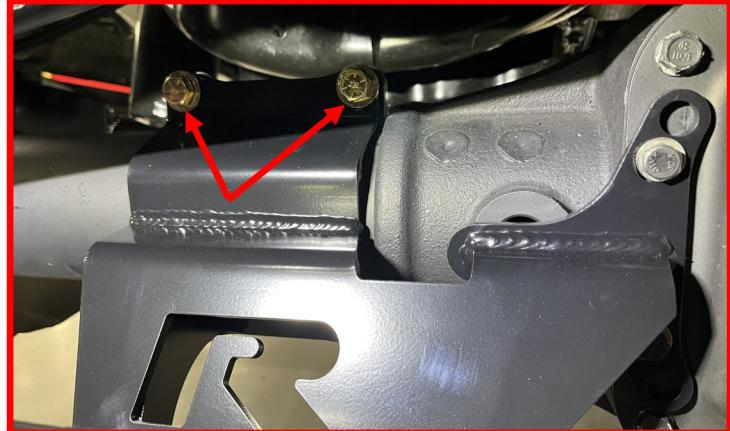
Tighten each of the four M10 nuts and bolts, making sure that the gap between each is approximately equal when tight. Tighten the M8 bolts on the differential.
