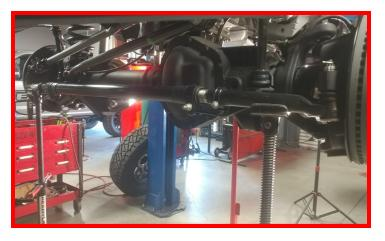
Unbolt the radius arm from the pivot point on the frame and raise the jackstands so the radius arm swings out of the way of the frame mount. Remove any aftermarket radius arm mount from frame location.
