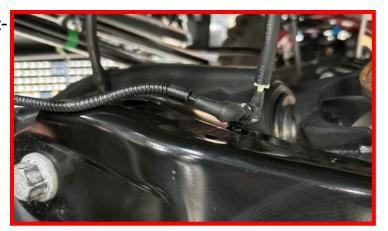
Remove factory radius arm from vehicle. Retain factory hardware.
