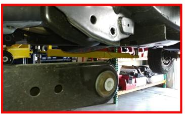
Remove vacuum lines from driver side factory radius arm.
