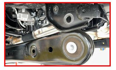
Install ReadyLift Radius Arm to axle using factory hardware for the upper connection and using the ReadyLift Cam Bolts for the lower connection. ReadyLift Logo should be facing toward the outside of the vehicle. Do not tighten at this time.
