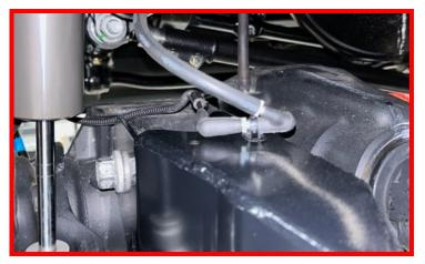
Torque the upper radius arm to axle bolts to 200 ft-lbs.
