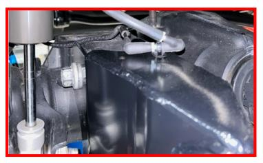
Lower the vehicle to the ground and torque the radius arm to frame connection to 200 ft-lbs.
