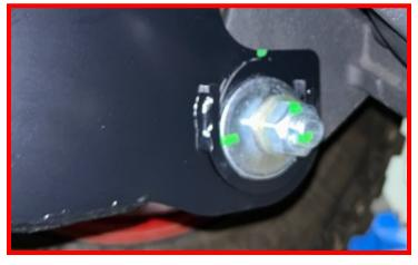
Install vacuum lines into holes on top of LH ReadyLift Radius Arm
