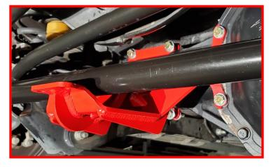
Using the supplied 7/16"x 2" long Hex Head Bolts, 7/16" flat washers and 7/16" top lock nuts, install the rear axle clam shell to the center stabilizer bracket, clamping both around the axle tube.
