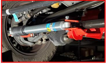
Using the M12 x 75mm bolts, washers and nut, install the driver stabilizer. Stabilizer body bushing should be installed with the stabilizer center link plate on top and the center stabilizer bracket on bottom of the stabilizer bushing (as shown in photo).
