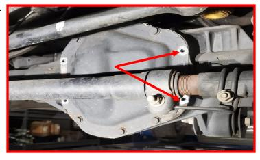
Differential ID tag shown installed on the drivers side using the (2) factory bolts.
