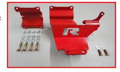
Install the center stabilizer bracket using the supplied 3/8" x 1-1/4" hex head bolts and 3/8" flat washers. Tighten bolts enough to secure the main body to the passenger side of the differential but do not tighten completely at this time.
