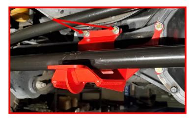
Tighten each of the four nuts and bolts making sure that the gap between each is approximately equal when tight.
