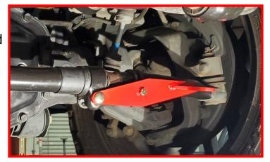
Install passenger side drag link bracket using the supplied M8 x 75mm hex bolts, M8 lock nuts, M10 x 90mm carriage bolts and M10 lock nuts. Do not fully tighten at this time.
