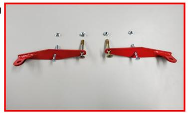
Note the orientation of the U-shaped clip on the rearward side, it will need to be reinstalled. Install the Driver and Passenger side shock mounts.
