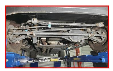
Remove the (2) middle bolts on the passenger side of the differential cover and retain the factory hardware. Save the differential ID tag for the step below.
