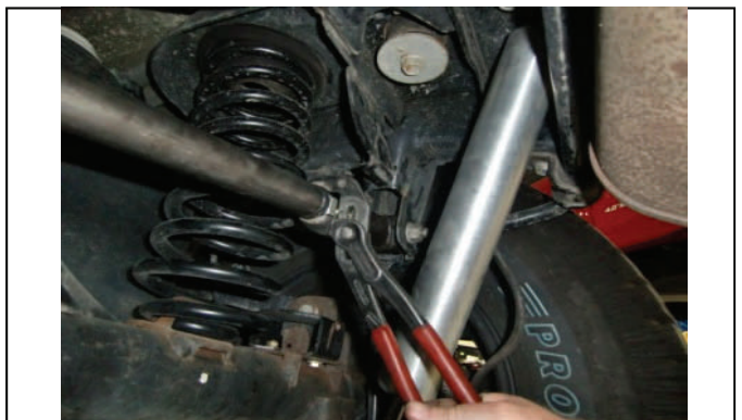
Adjust track bar under rear of vehicle and tighten jam nuts.
