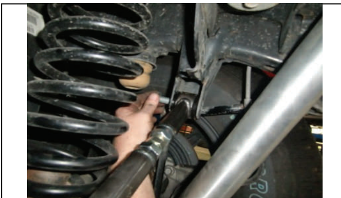
Reinstall adjustable track bar in reverse of removal steps.
