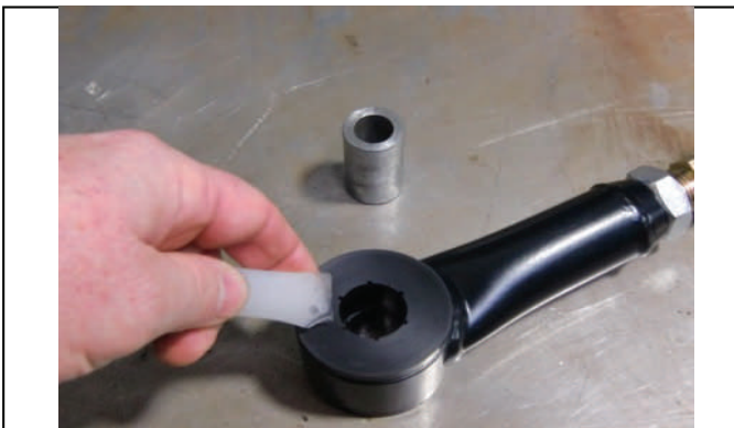
Use assembly lube on bushings and sleeves.
