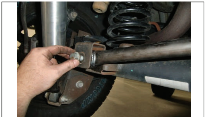
Straight zerks goes on short end and 90 degree on longer end
