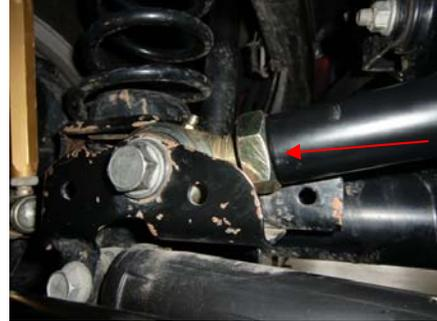
Once the desired length is reached you must tighten and set the jam nut on the adjustable end of track bar.
