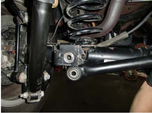
Re-install new track bar.
