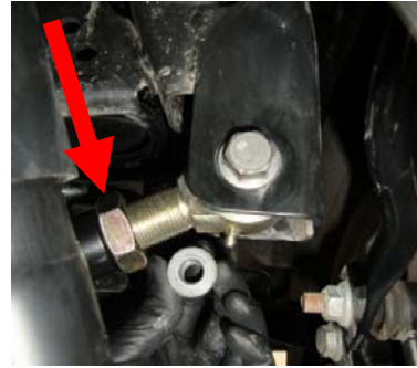
Once the Desired Length is reached you must Tighten/ Set the jam nut on the adjustable end of track bar.
