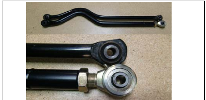
Place track bar side by side to pre set the length. The length will vary depending on your application.
