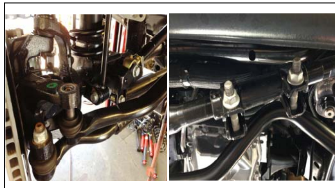
4. Remove the steering drag link from the axle, then loosen the coupler.
