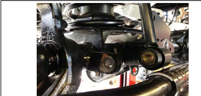
7. Remove the sway bar end links from the axle.
