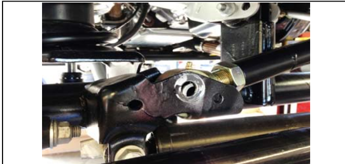
8. Remove the track bar from the axle side.
