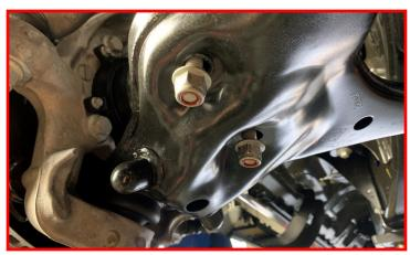
Loosen and remove the lower control arm pivot bolts. Retain the factory bolts.
