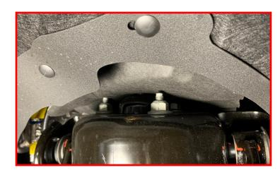
Remove the lower strut nuts. Retain the factory mounting hardware.
