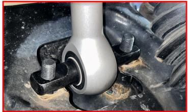
Install the supplied M12 lower strut nuts.
