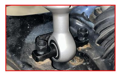
Using an appropriate jack, carefully jack the lower control arm into the frame side pivot pockets. Install the factory pivot bolts.
