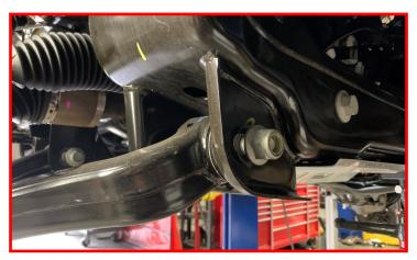
Remove the lower control arm pivots from the frame side pivot pockets.
