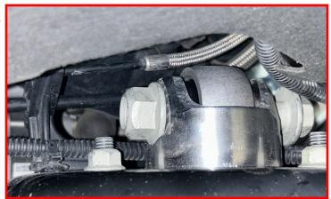
Continue to raise the lower control arm up until you are able to install the supplied M12 bolts and washers.
