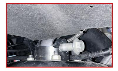
Install supplied M16 locking flange nut onto the coilover mounting bolt.
