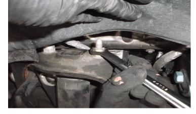
Install the provided shocks to the frame using the provided hardware that came with the shocks.
