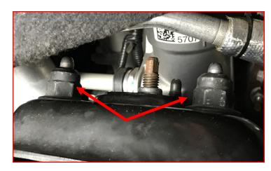
Install the coilover into the top hat using the supplied M16 Flange bolt and M16 locking flange nut.
