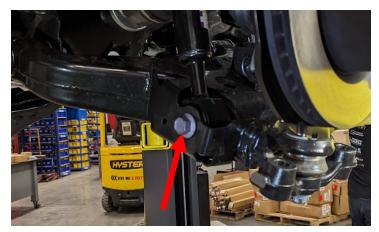
Allow the lower control arm to swing out of the way.
