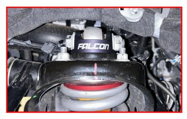
Raise the lower control arm back up, while installing the sway bar end link into the control arm pocket.
