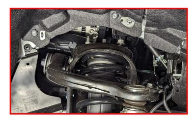
Remove lower control arm to strut bolt. Remove strut from vehicle.
