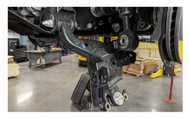
Remove the four (4) upper strut bolts and remove strut from vehicle.
