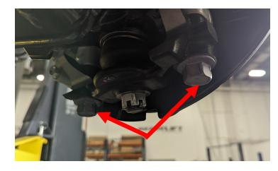
Remove lower control arm to strut bolt.
