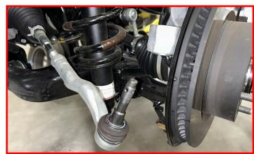
Remove the four (4) upper strut nuts.
