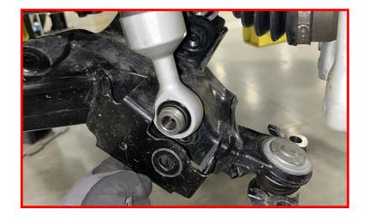
Install the factory lower shock bolt.
