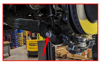
Install the lower ball joint cradle into the knuckle using factory hardware.
