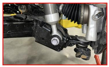
Install the lower strut bolt and nut.
