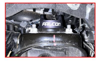
Install Falcon coilover assembly into Falcon top hat. Insert M16 bolt into the top hat and through the top of the coilover.
