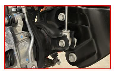
Install the front wheels. Lower the vehicle to the ground. Torque the lug nuts to the wheel manufacturers specs. Jounce the vehicle a few times to settle it to the new ride height. Torque the lower shock hardware to 65 ft-lbs.
