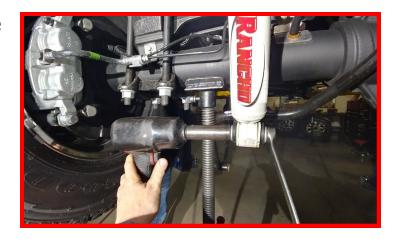
Install rear Falcon shock using factory hardware.
