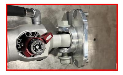
Install the coilover using the supplied M12 flange nuts on the upper mount.
