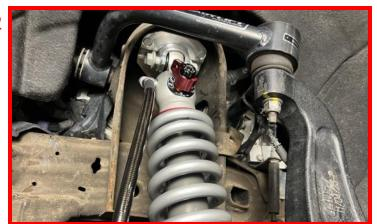
Using the supplied M10 bolts and flange nuts, secure the off-set bar pin to the lower control arm.
