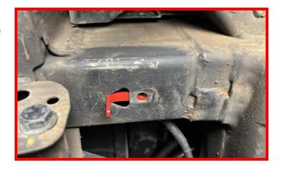
Attach the reservoir to the frame using the factory M8 splash guard bolt and supplied nut plate.
