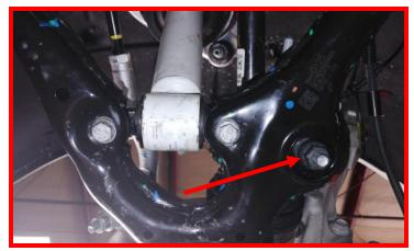
Remove the outer tie rod end to the knuckle using factory hardware.
