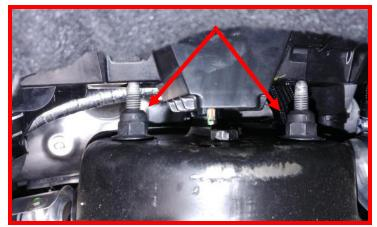
Install the top hat to the falcon coilover using the supplied M16 bolt and nut.
