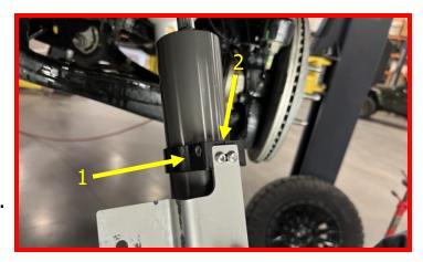
Remove the clip nut from the frame and insert the supplied nut plate through the triangle hole in the frame. Align the nut above the round hole in the frame.
