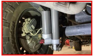
Install the rear wheels and lower vehicle to the ground. Torque the lug nuts to the wheel manufacturer specs and all shock hardware to 65 ft-lbs.
