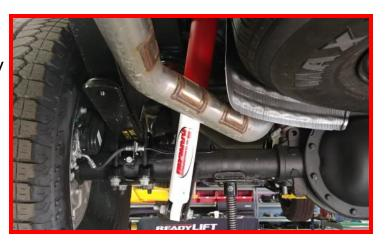
Install the Falcon shocks using the factory hardware as shown.
