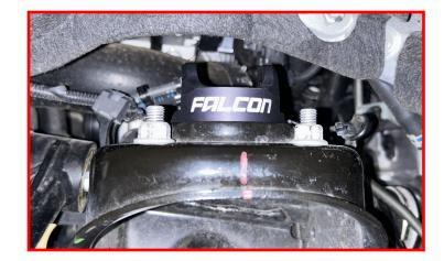
Install Falcon coilover assembly into Falcon top hat. Insert M16 bolt into the top hat and through the top of the coilover.
