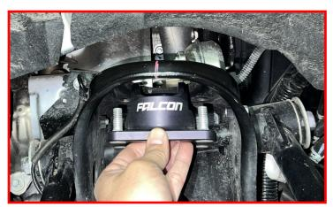
Install the provided M10 hardware Torque nuts to 40 ft-lbs.
