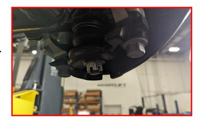
Loosen but do not remove the (4) top strut nuts.
