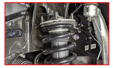
Install Falcon Front Strut top hat into the strut tower.
