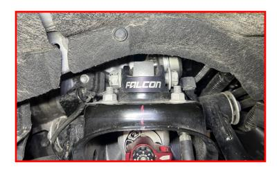
Raise the lower control arm back up, while installing the sway bar end link into the control arm pocket.
