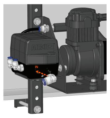
Route the supplied 3/8" air line from the 3/8" PTC elbow (above) to the 3/8" PTC Boost Tank fitting. Use the supplied zip ties to properly secure the air line while avoiding hot exhaust and sharp edges. Use the air line cutter supplied with your  $AirlQ^{TM}$  system, or a sharp razor blade to make clean square cuts to the air line.
