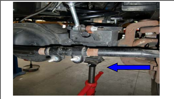
Raise axle to engage spring and shock mount.
