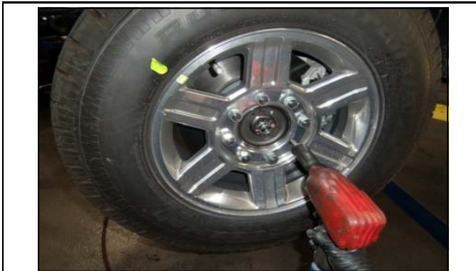
Raise front end of vehicle, support frame & remove wheels.
