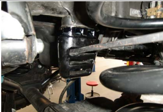
Install new bump stop. Use pry bar to press into frame.
