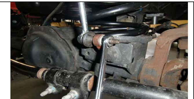
Re-attach sway bar to axle.
