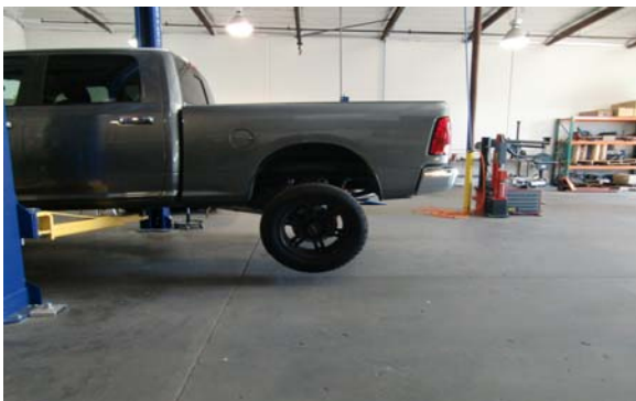
Raise rear of vehicle on level ground and support frame.
