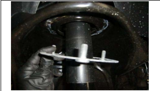
Remove factory retainer plate & nuts.
