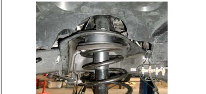
Install ReadyLIFT Coil Spacer.
