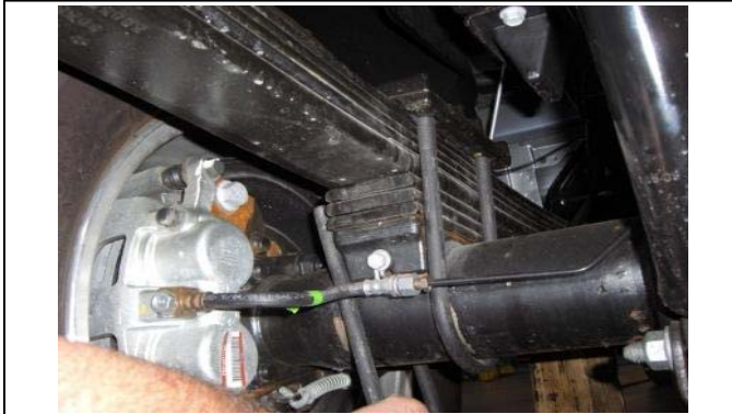
Disconnect U-bolts and remove, one side of vehicle at a time.
