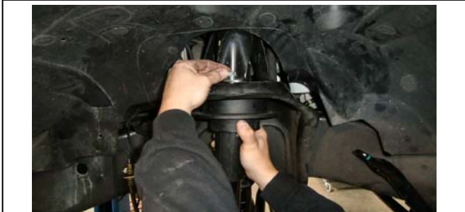
Attach ReadyLIFT Coil Spacer with supplied M10 serrated flange nuts "Leave Loose".
