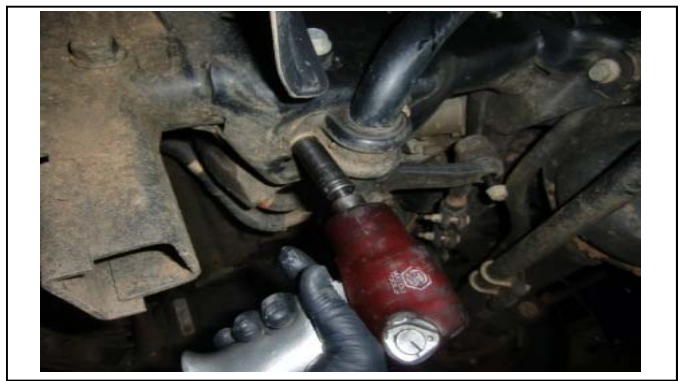
Disconnect sway bar from frame.
