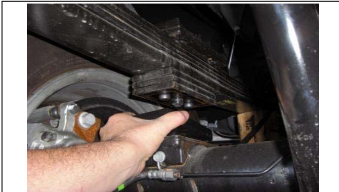
Place new lift block on axle pad, center pin down.
