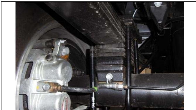
Install new u-bolts & hardware, reattach shock and tighten.
