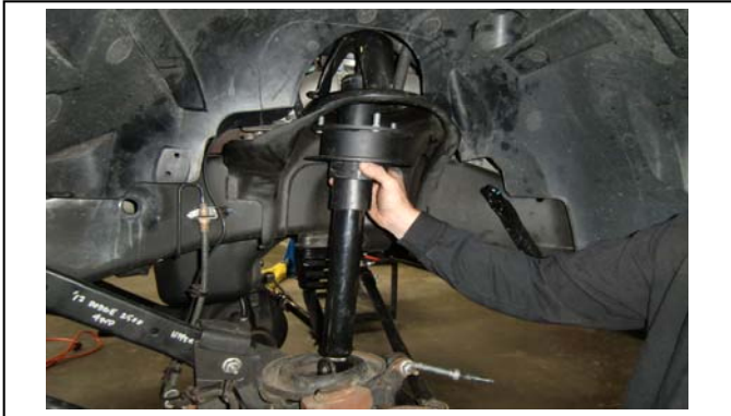
Install ReadyLIFT Coil Spacer.
