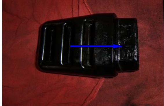
Grease top of new bump stop.
