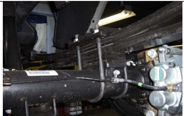
Support axle & disconnect lower shock mounting hardware.
