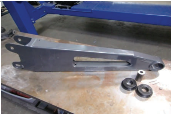
Photo shows one side Stage 2 radius arm and bushing kit
