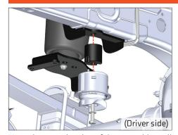
Move the upper bracket of the assembly until the lower hole lines up with the bumpstop bolt hole in the frame.
