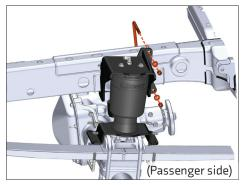
Fasten the U-bolt to the upper bracket with the supplied flat washers and nuts. Leave the assembly loose until the bumpstop spacer has been installed in the lower hole of the bracket.
