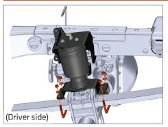
spring, then mount the lower bracket to the leaf springs using the supplied smaller 3/8" U-bolts, flat washers and nuts.
