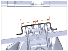
Apply downward force to extend the air Make sure that the lower bracket is centered Repeat for passenger side. over the U-bolt saddle and snug the nuts.
