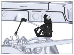
If your truck is equipped with the rear height Unbolt factory bumpstops using a 13MM socket. sensors shown, you must purchase 88-21150-1 to complete installation of this kit.
