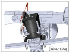
Mount the air spring assembly upper bracket to the frame with one of the supplied 3/8" U-bolts. The U-bolt should slip between the back of the frame and any factory hoses or wiring.
