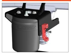
Install the E-brake relocation bracket on the driver side upper bracket using the supplied 1/4" hardware.
