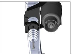
Slip the bump stop into the cup on the provided bump stop spacer.
