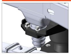
provided 3/8" Grade 8 hardware into the bump snug the two 3/8" bolts. stop spacer as shown.
