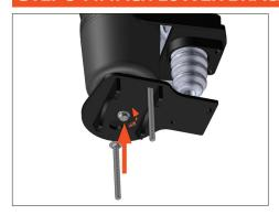
Install the 3/8" carriage bolts into the holes on the lower bracket, then apply downward force to extend the air springs and bring the lower bracket near the axle.
