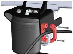
Route the E-brake cable through the middle of the base bracket. Secure the cap piece of the bracket to the base with the other two 1/4" screws (longer of the two goes in the top hole) to capture the E-brake cable.
