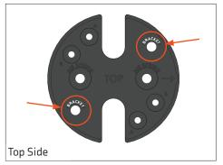
For the final spacer in your stack, place a 3/8"-16 nut in the two hex holes on the underside of the lift spacer that correspond to the holes marked "BRACKET" on top of the lift spacer.
