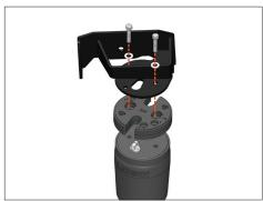
Bolt one lift spacer between the air spring and upper bracket using the "AIR SPRING" holes and supplied 1.75" long 3/8" bolts with flat washers. Apply some threadlocker to each bolt.
