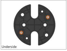
Place a 1/4"-20 nut in the two hex holes on the underside of the lift spacer that correspond to the holes marked "B" on top of the lift spacer.
