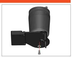
Unless installing a 1" lift, remove the one 3/8" bolt holding the lower bracket to the air spring and remove from vehicle.
