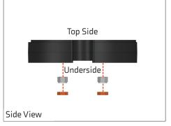
Press a 1/4" hex spacer in the two hex holes, on top of the nuts, as shown. This will secure the nuts in the hex holes.
