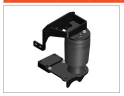
Fully deflate air springs and disconnect air line from the air fitting.
