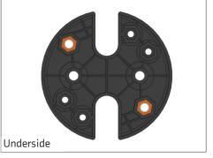
Press a 3/8" hex spacer in the two hex holes, on top of the nuts, as shown. This will secure the nuts in the hex holes.
