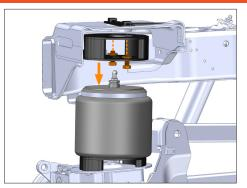
Carefully separate the air spring from the upper bracket and compress the air spring by pushing down on it.
