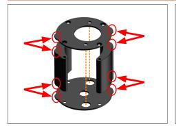
The two plates of the upper bracket should be oriented so the 1/2" holes on the upper plate line up with the clearance holes on the lower plate.
