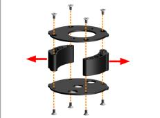
Using a 3/16" hex socket, un-bolt the 8 fasteners holding the upper bracket together.
