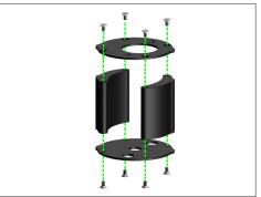
Fasten the upper bracket together with the supplied 5/16" hardware.
