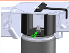
Re-install the hairpin clip in the groove of the air spring.
