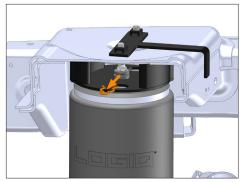
Fully deflate air springs and disconnect air line from the elbow air fitting.
