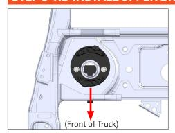
Ensure the upper bracket is in the orientation **(B)** Re-install the two 1/2" bolts with some shown before installing the bolts.
