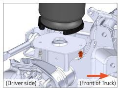
Press down on the lower bracket to bring it in contact with the axle perch.
