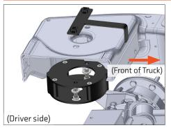
Place the weld nut bracket on top of the crossmember, with the bent tab facing the front of the truck, and line it up with the two holes shown.
