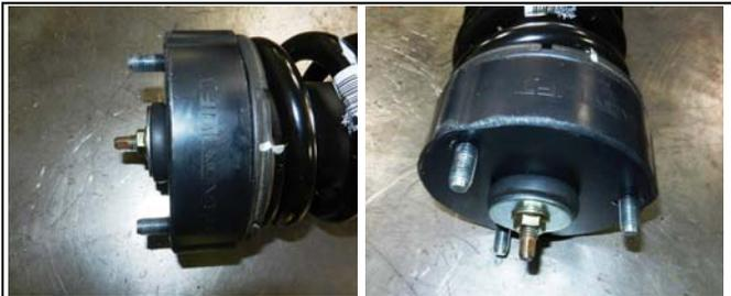
Install the rubber isolator and ReadyLIFT top hat spacer onto the strut using a supplied washer and gold 10mm x 1.5 flange nut. Use a 15mm and 6mm wrench. Make sure to line up the markings from top to bottom on the strut. **Do not use an impact gun, tighten down by hand.**
