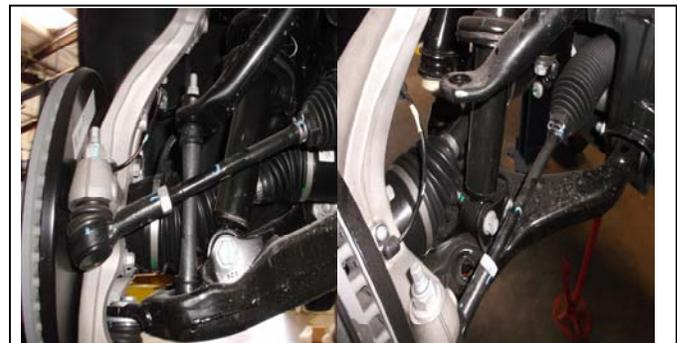
4. Remove the sway bar end links from the vehicle. Using a 15mm socket on top and a 13 mm socket on bottom.
