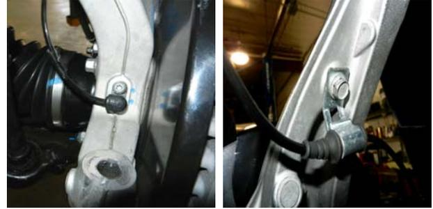
6. Remove the ABS line from the knuckle using a T30 torx socket and a 10mm socket.
