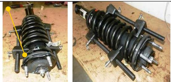
12. Mark the back side of the strut (frame side), on the top and bottom for aid in reinstallation alignment. Use a strut spring compressor to compress the spring.
