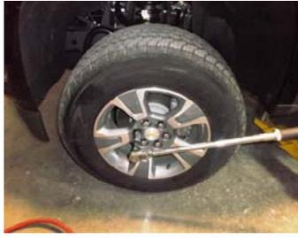
Reinstall the wheels using a 22mm socket, lower the vehicle to the ground and torque the lug nuts to 100 ft lbs. Tighten down the lower control arm bolts using a 24mm socket if loosened.
