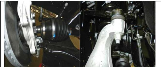
Reinstall the axle into the steering knuckle. Reinstall the upper control arm to the steering knuckle. Torque down using a 18mm socket. Install the factory hardware to the axle and tighten down with a 36mm socket.
