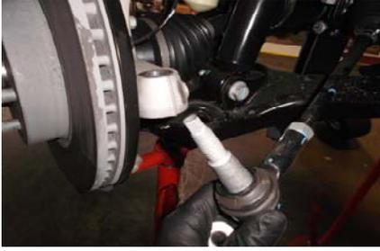
5. Remove the tie rod ends from the steering knuckle using a 21mm socket.
