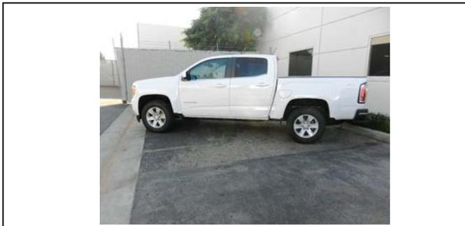
Put the vehicle onto level ground. Measure from the ground to the center of the fender well at all four wheels. Record the data in 1.
