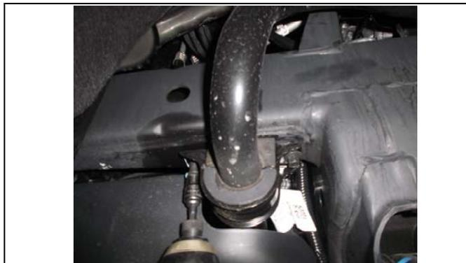
3. Loosen the factory sway bar at the frame using a 10mm socket.
