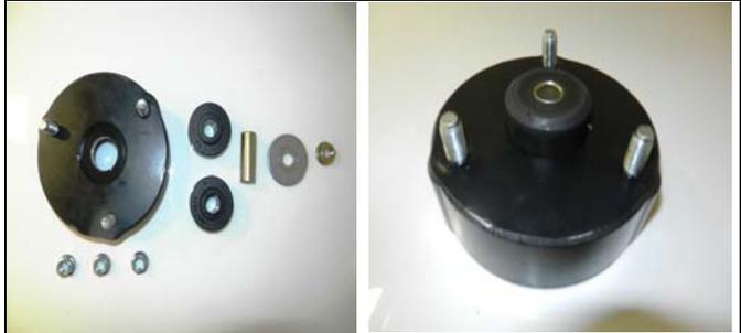
Install the rubber bushings to each side of the spacer. Lube the metal sleeve and press into the bushings.
