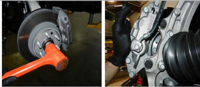
7. Unbolt the axle nut using a 36mm socket. Use a soft mallet or press tool to knock the axle from the knuckle. Remove the brake calipers from the knuckle using a 18mm socket. Hang out of the way.
