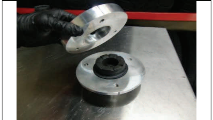
Place OE strut bushing between two halves
