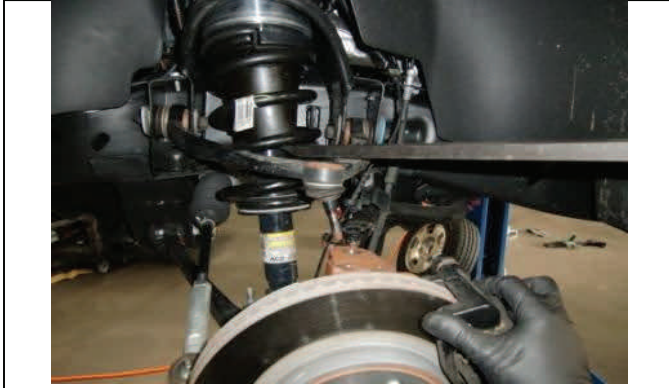
Raise suspension to reconnect ball joint to spindle
