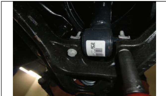
Remove lower strut mounting bolts
