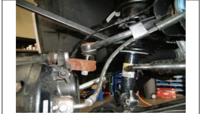
Use a pry bar to depress ball joint into spindle, attach nut
