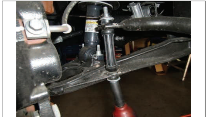
Reconnect sway bar end link and ABS/brake brackets
