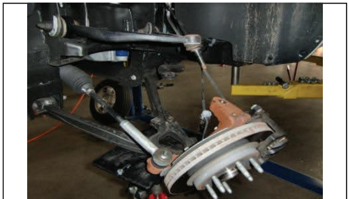
Lower suspension and remove strut assembly from vehicle
