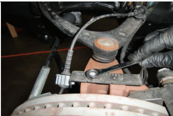
Disconnect ABS bracket on spindle
