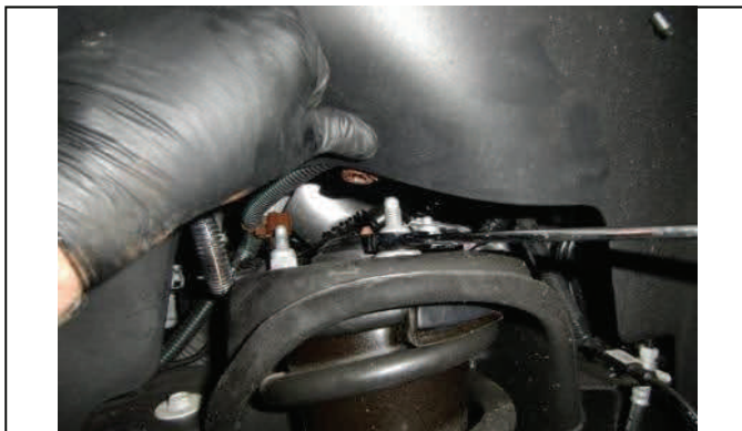
Remove upper strut mounting nuts
