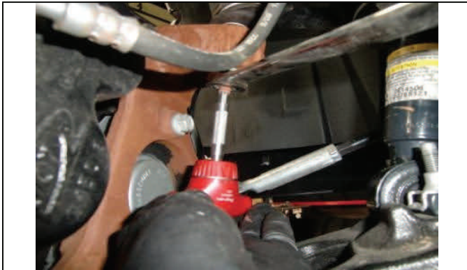
Tighten to spec, use allen wrench to hold ball joint stem
