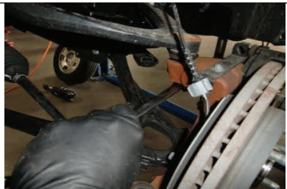
Loosen upper ball joint nut
