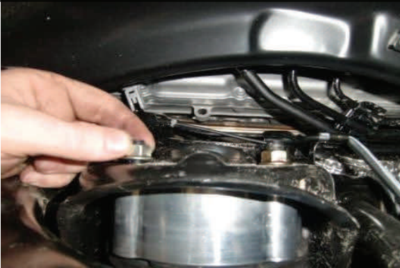
Reinstall strut using provided hardware on top, OE on lower
