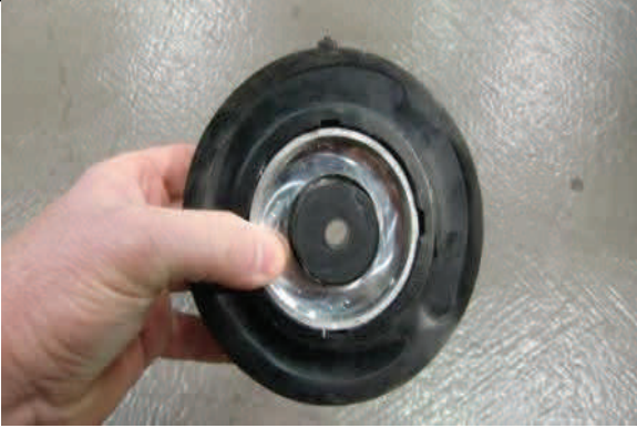
Place OE shaft bushings in original locations as shown
