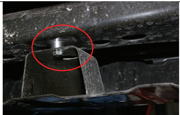
Install (2) skid plate spacers with new hardware
