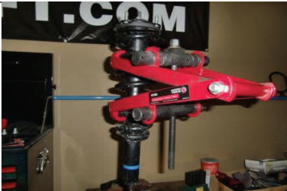
Use appropriate spring compressor for strut disassembly
