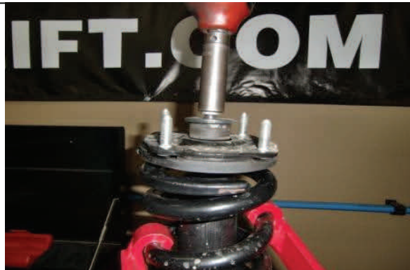
Remove retaining hardware, set aside, it will be reused
