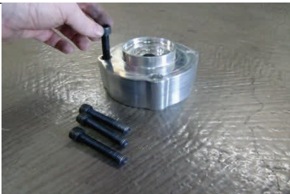
Install provided bolts into T6 billet spacer countersunk holes
