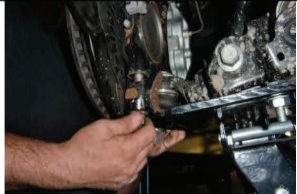
Use a jack, attach lower ball joints bolts, start by hand
