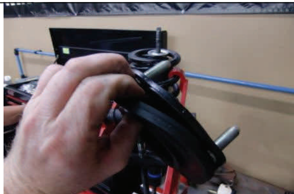
Remove OE upper spring isolator
