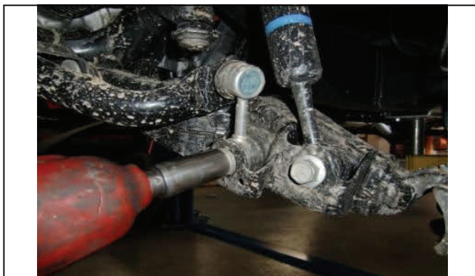
Disconnect lower sway bar end links
